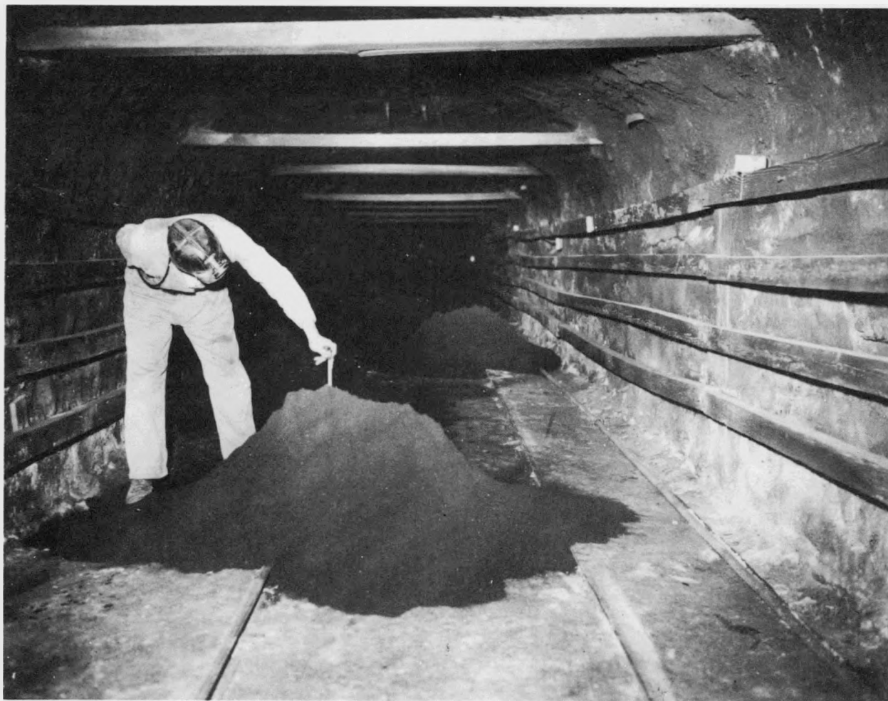
FIGURE 11. - Dust heaps on mine floor for explosion test.
