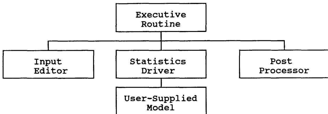
Figure 2. Structure of the SUNS Software Package
