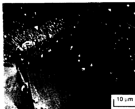
Fig. PA-4. Tantalum deformed at higher strain-rates does not show preferential attack; the features shown are indicative of embrittlement.
