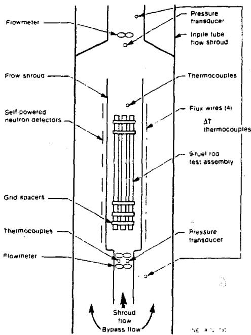
Fig. 1 Schematic representation of the Test PCM-5 test train assembly showing the relative positions of the fuel rods and train instrumentation.
