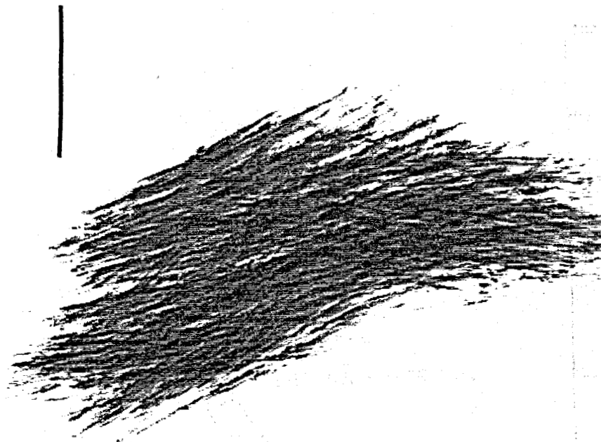
Figure 13a. Sepiolite fibers in the starting clay; scale: 1.0 micron.
