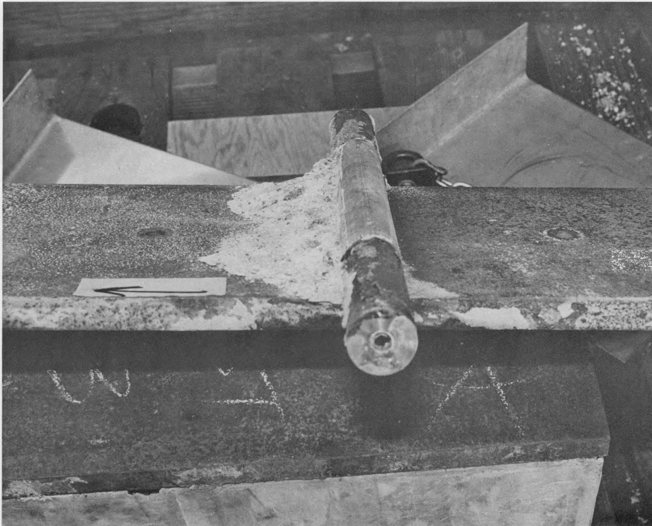
Fig. 7. Cooling tube/concrete damage after monotonic test, specimen 3 (1-in. Schedule 40)
