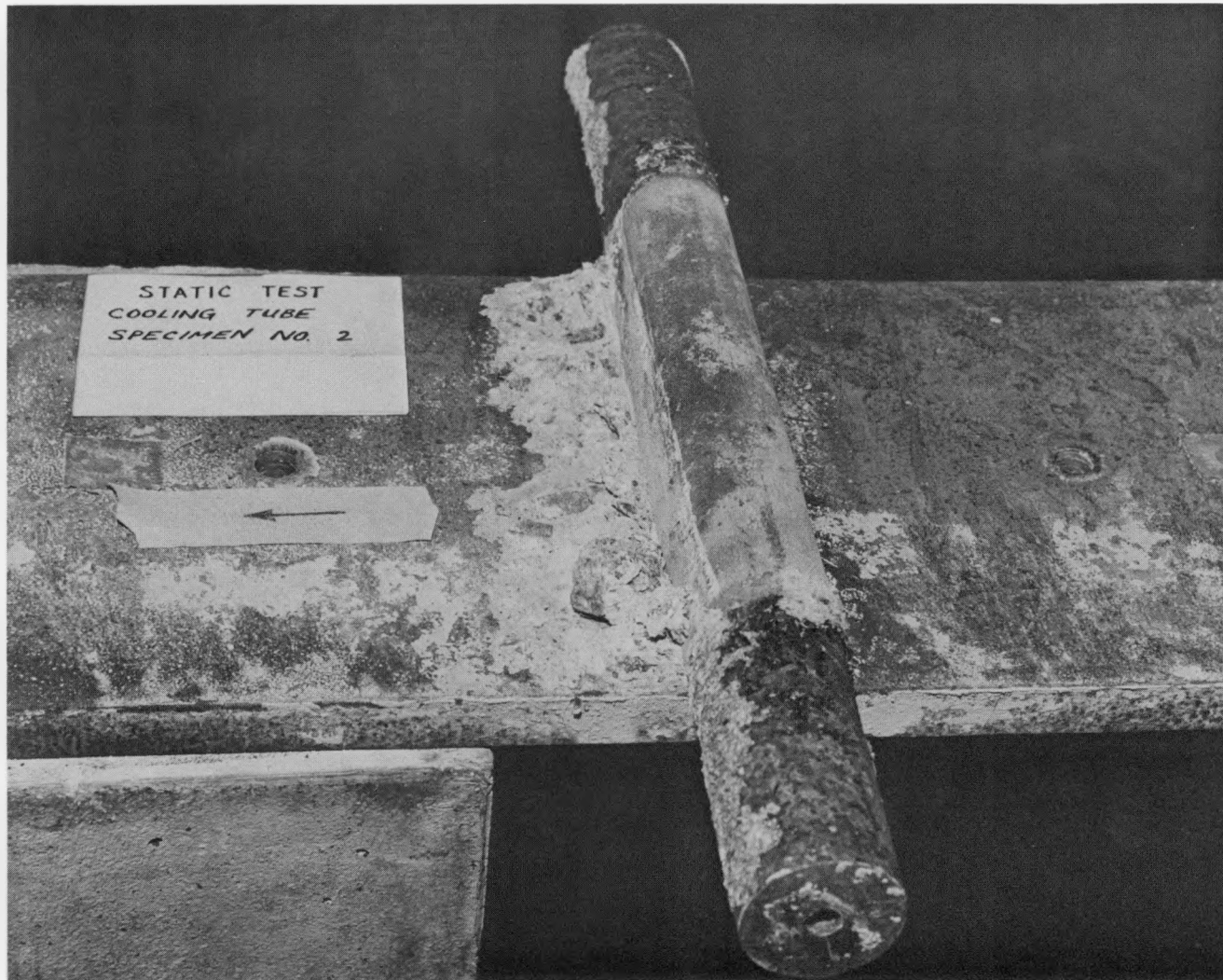
Fig. 11. Round tube distortion after monotonic test, specimen 2 (1-1/4-in. Schedule 40)
