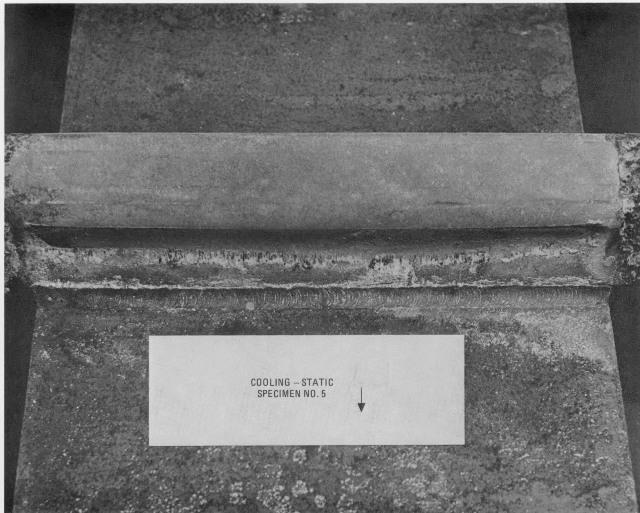
Fig. 13. Square tube distortion after monotonic test, specimen 5
