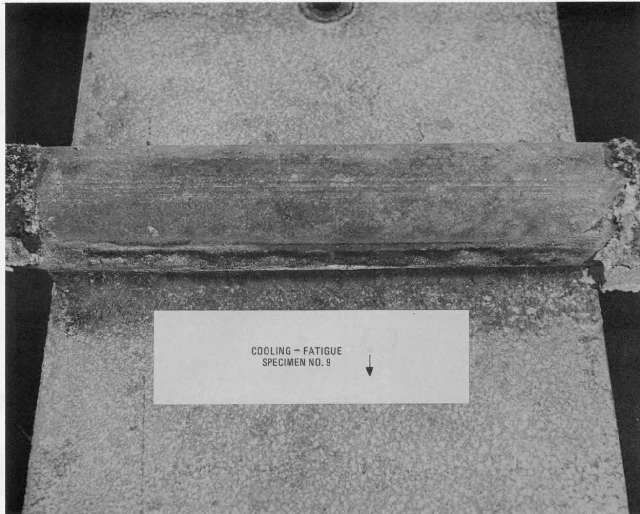
Fig. 29. Round tube distortion after cyclic and monotonic test, specimen 9 (1-1/4-in. Schedule 40)
