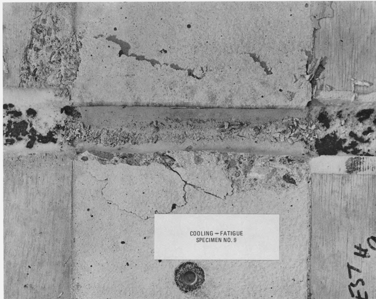
Fig. 30. Concrete damage after cyclic and monotonic test, specimen 9
