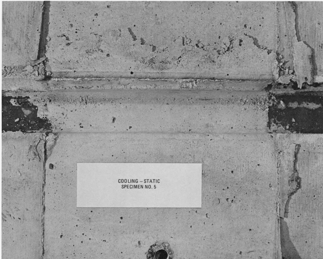
Fig. 14. Concrete damage after monotonic test, specimen 5 (1-1/2-in. square tube)
