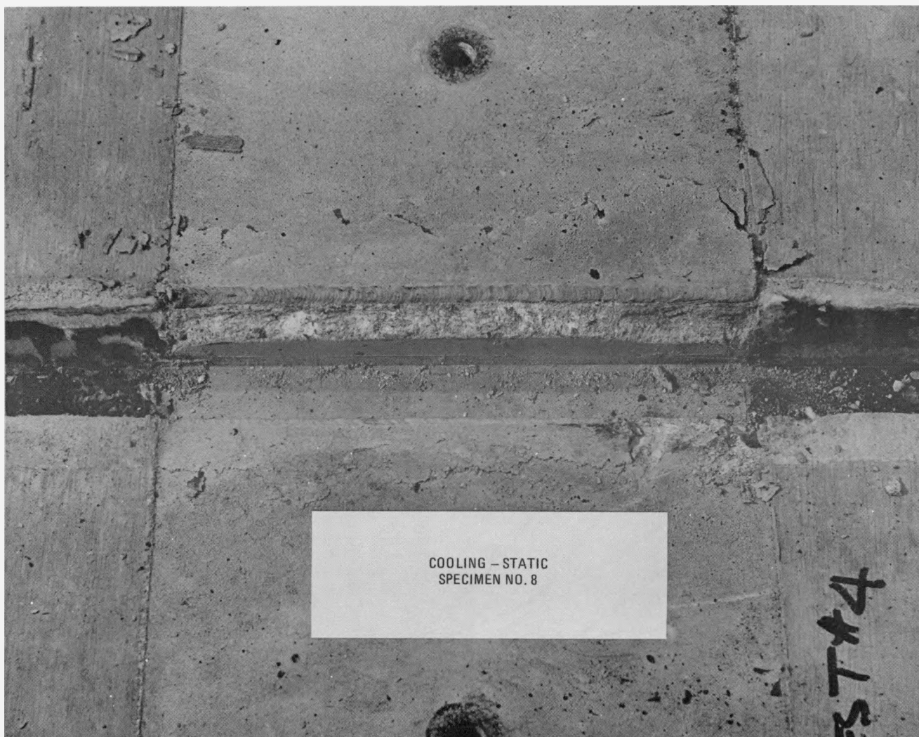
Fig. 18. Concrete damage after monotonic test, specimen 8 (1-1/4-in. square tube)
