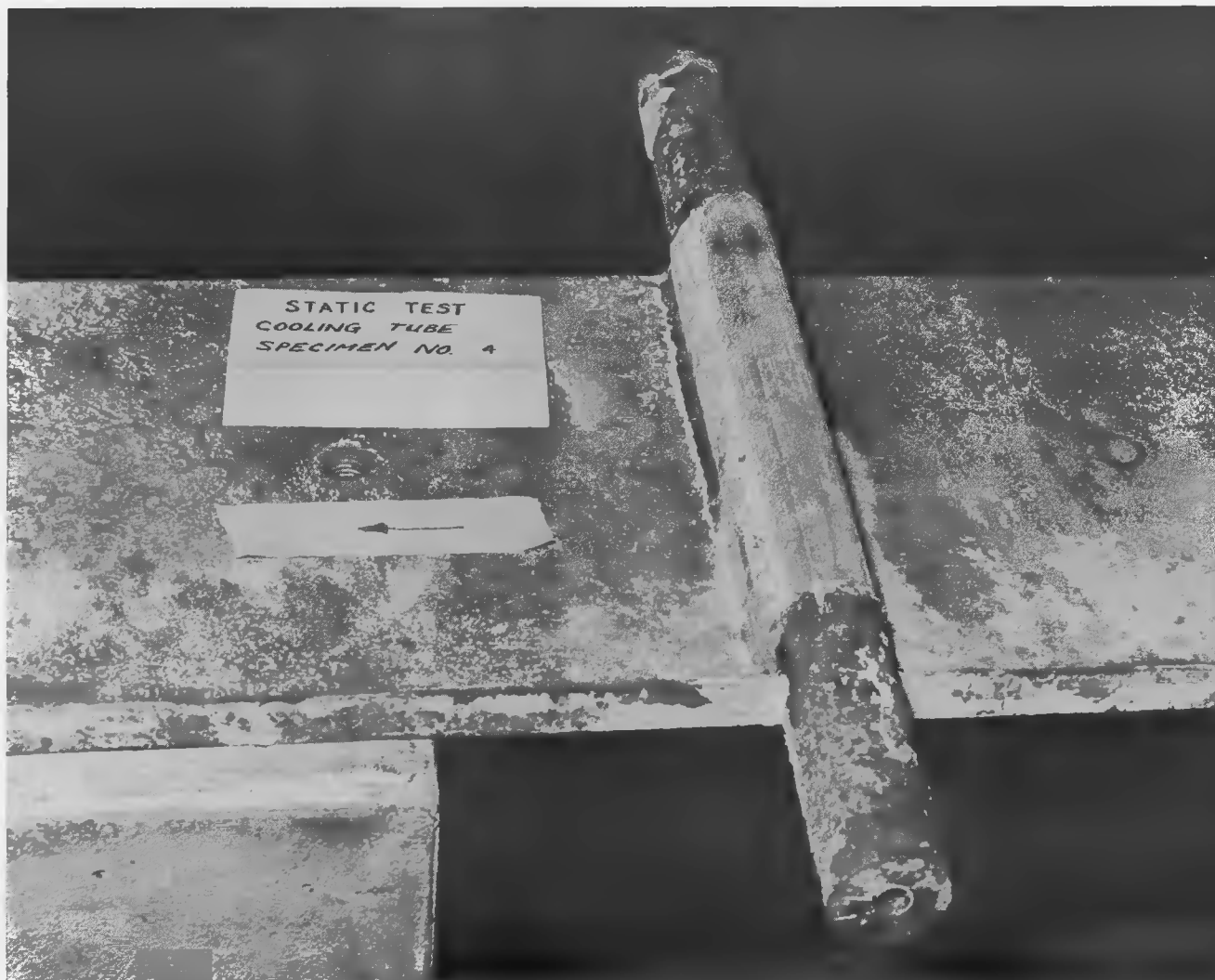
Fig. 9. Round tube distortion after monotonic test, specimen 4 (1-in. Schedule 40)
