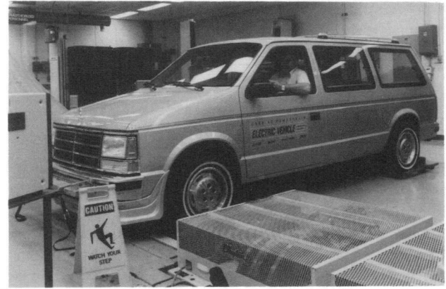
Figure 9: Dynamometer Testing of DSEP
