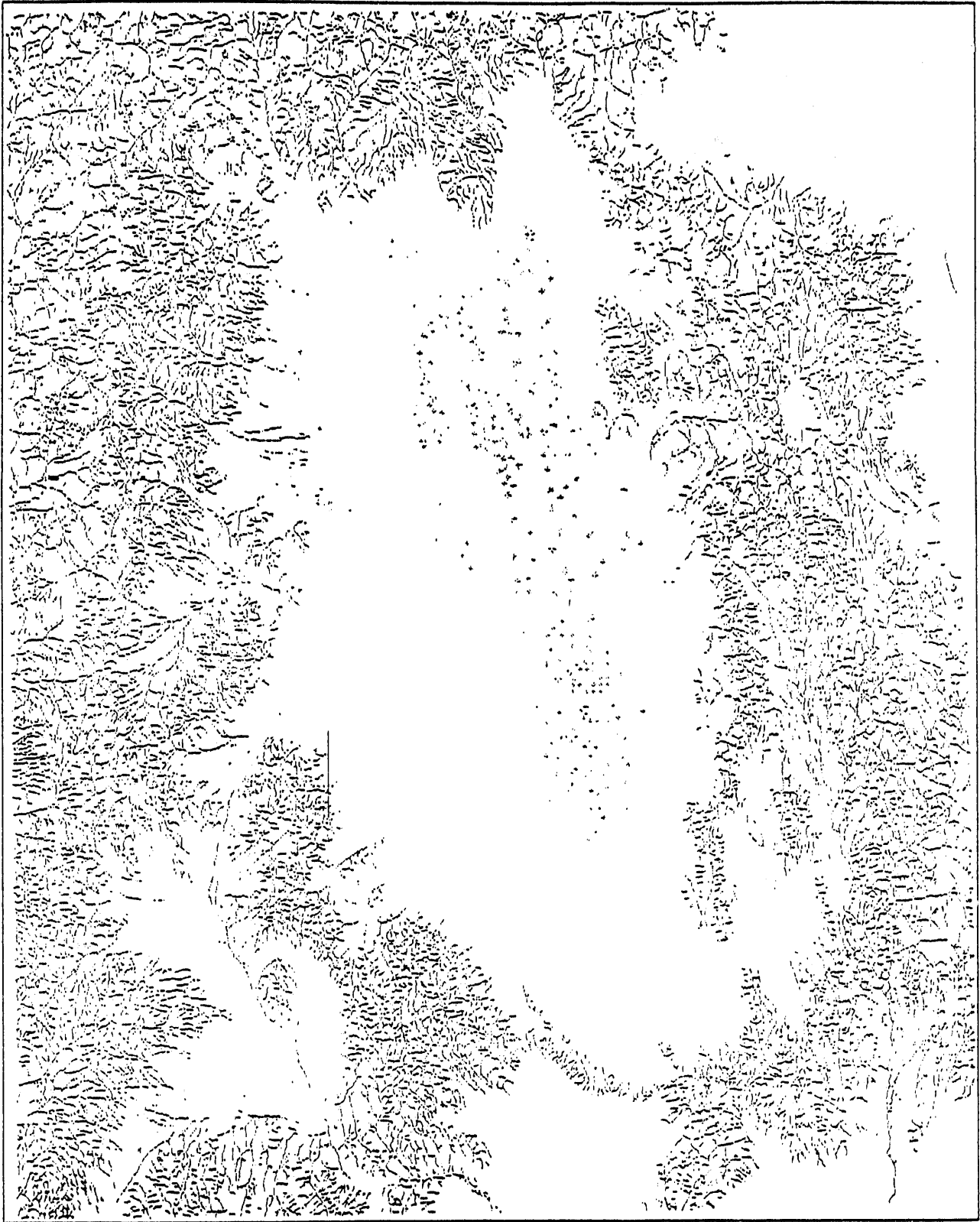
FIGURE 11. Low-Point Strings Detected in the Yucca Flat Study Area DEM by the RGA Valley Algorithm
