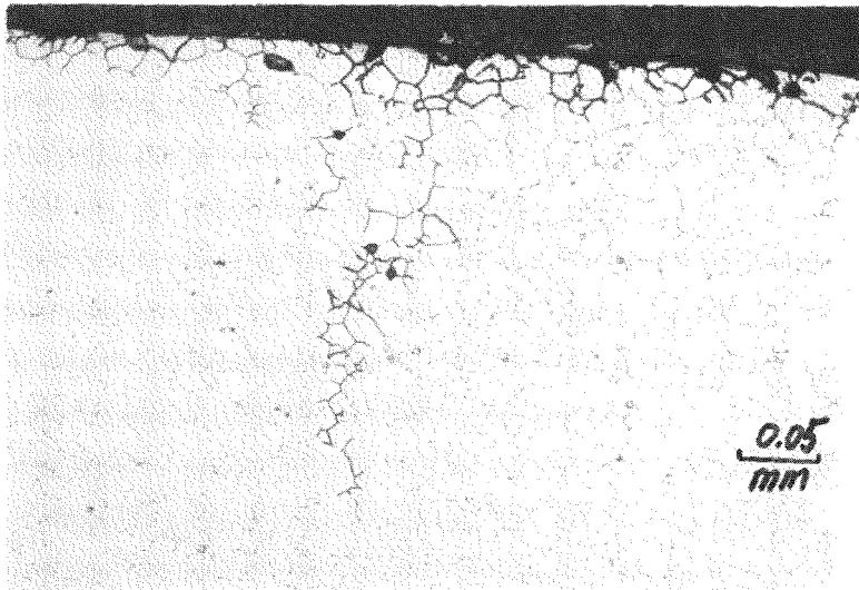
Specimen No. 32 0.025 mm = Uniform IGA 0.30 mm = SCC max.
