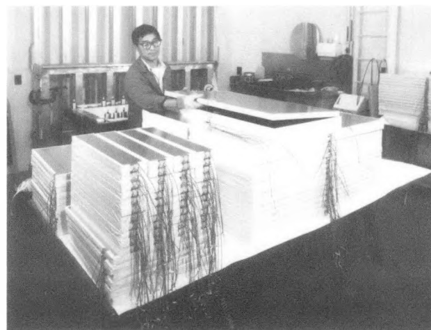
Figure 15. Large-area heat-flow meters for use in MoWiTT. (CBB 828-7550)
