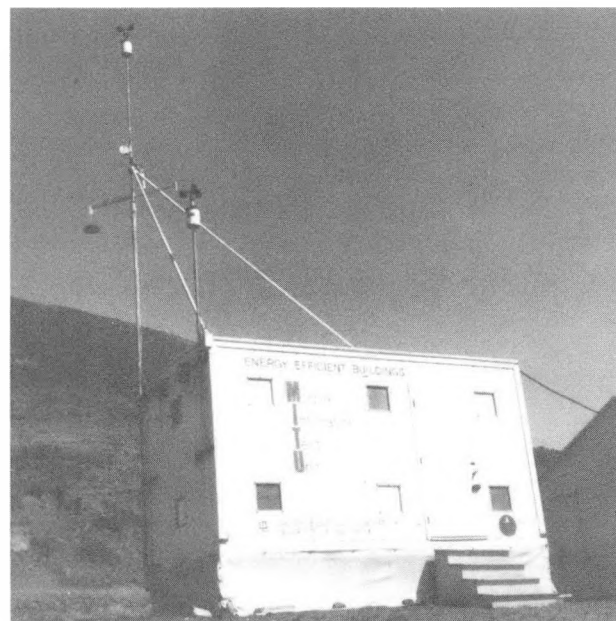
Figure 2. The Mobile Infiltration Test Unit at a site near Fort Cronkhite, CA. (XBB 810-9909)
