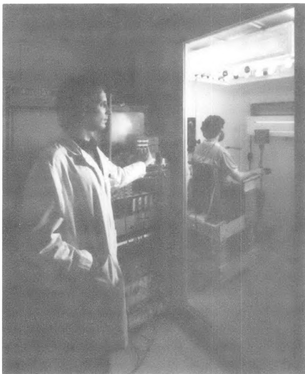
Figure 5. A view of the isolation chamber used to test the effects of lights upon human subjects. (CBB 828-7259)
