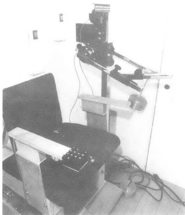
Figure 6. Close-up view of the test chair; apparatus to left of chair measures muscle strength. Subject uses keyboard in right armrest to perform visual tasks. (CBB 828-7370)
