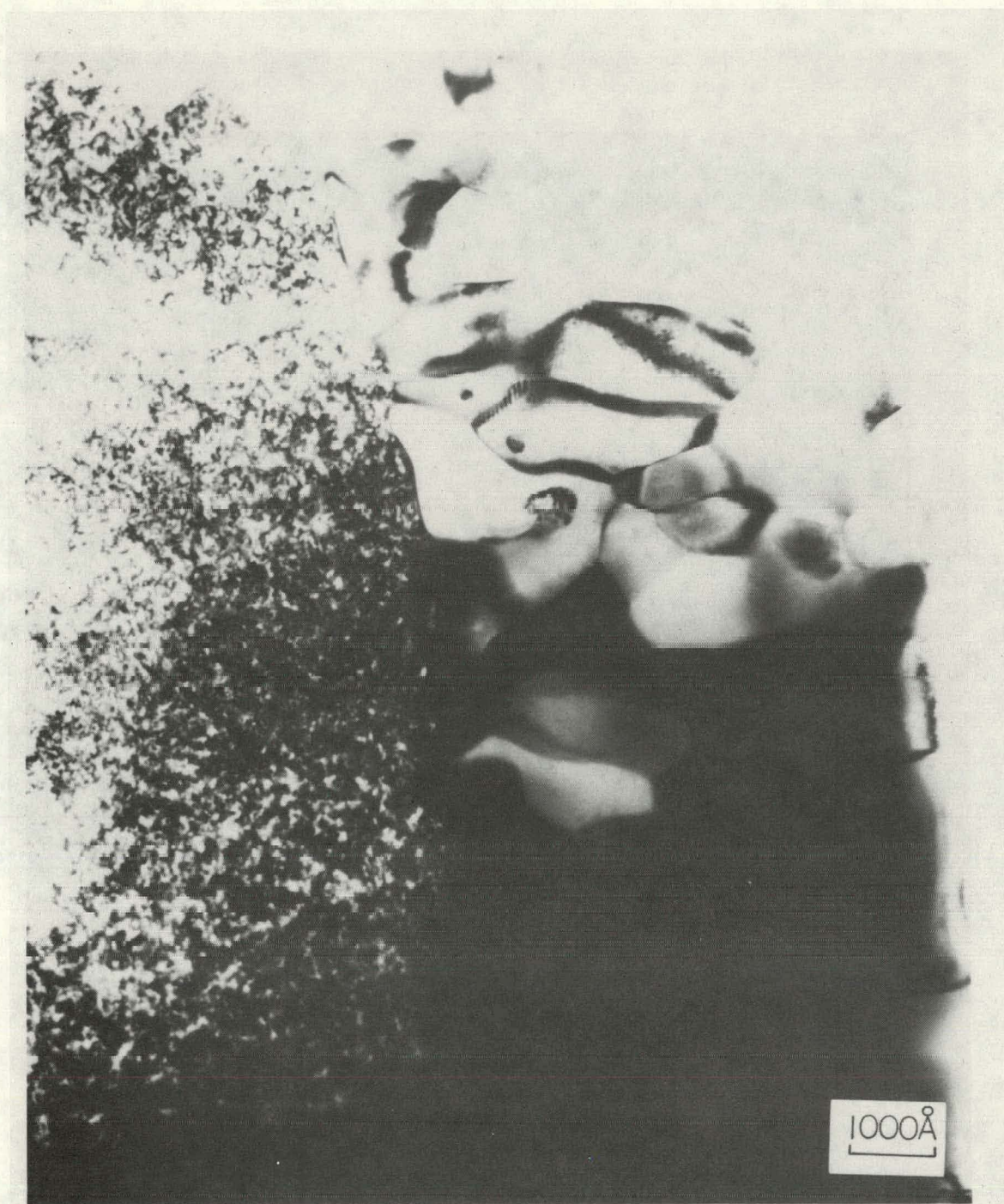
Figure 5. The corresponding bright field micrograph of Fig. 4 showing the columnar nature of the Al 5 grains near the Nb interface.
