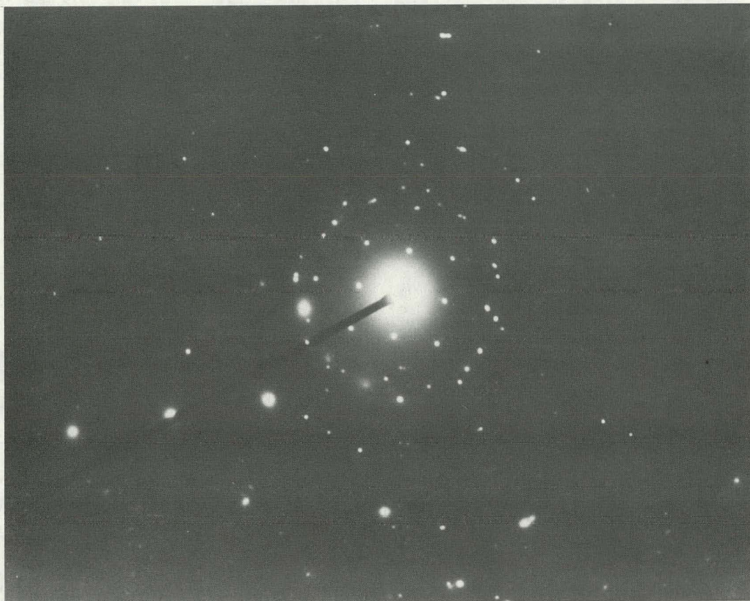
Figure 4. The selected area electron diffraction pattern of the boundary region between the Al 5 and the residual Nb. The square pattern near the center maximum is the (001) Al 5 zone axis pattern and the BCC (111) is represented by the brightest diffraction spots.
