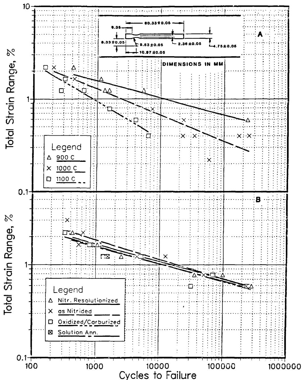
Figure 1. Reverse Bend Fatigue Test Results, for Inconel Alloy 625:
