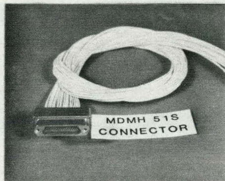
FIGURE 3. Cable Prepared for Electrical and Mechanical Tests
