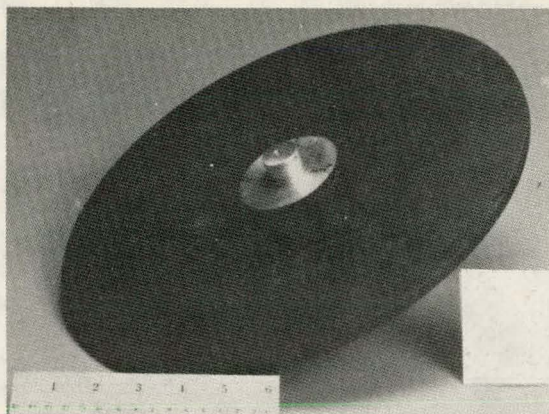
Fig. 6. Constant-Thickness Graphite/Epoxy Quasi-Isotropic Composite-Laminate Rotor.
