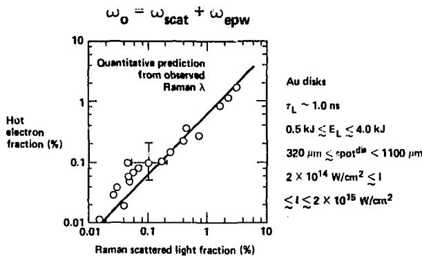
FIG. 5. For gold foils, the electron/ion collision frequency is comparable to the SRS growth rate and allows collisional damping to greatly reduce the stimulated Raman scattering.
