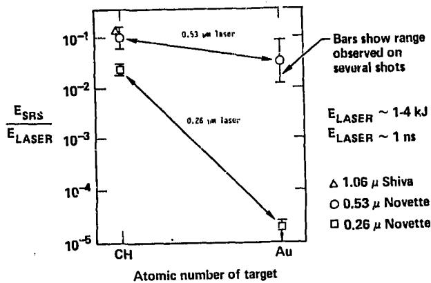
FIG. 6. Summary of laser plasma experiments with gold disks. Target coupling is very favorable at short wavelengths.
