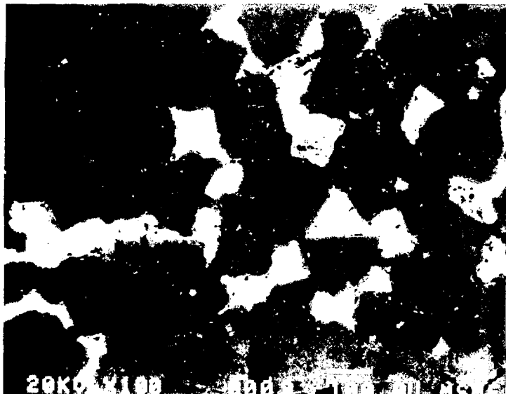
Figure 2. Typical serial section of Berea sandstone. The rock is composed mainly of quartz grains (dark gray), feldspar grains (medium gray), and products of grain dissolution (light gray). The pore space is impregnated with Wood's metal alloy (white), and epoxy (black). [XBB 908-6348]
