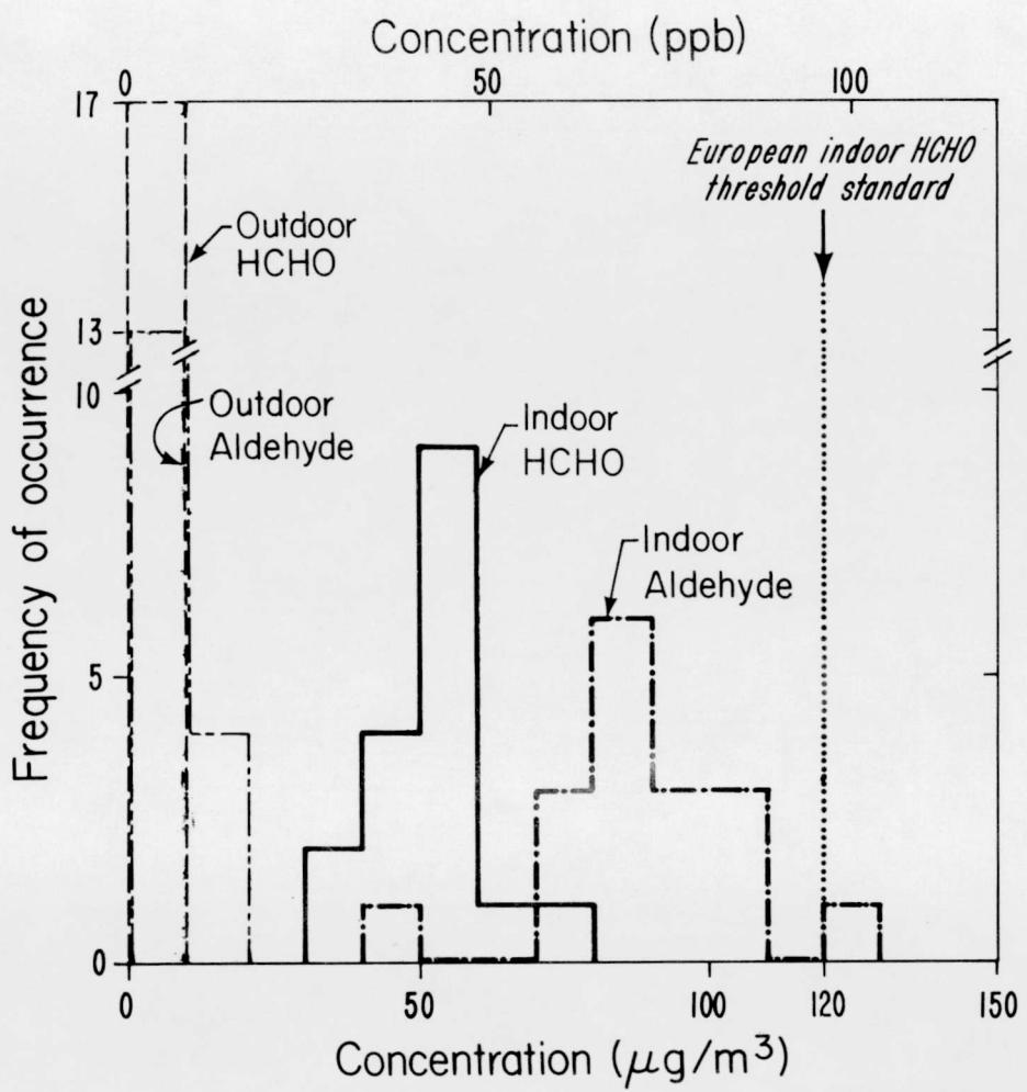
Figure 3. Histogram of indoor and outdoor formaldehyde and total aliphatic aldehyde concentrations in the Iowa State University Energy Research House, December, 1978. The house has an air exchange rate of about 0.2 ach.
