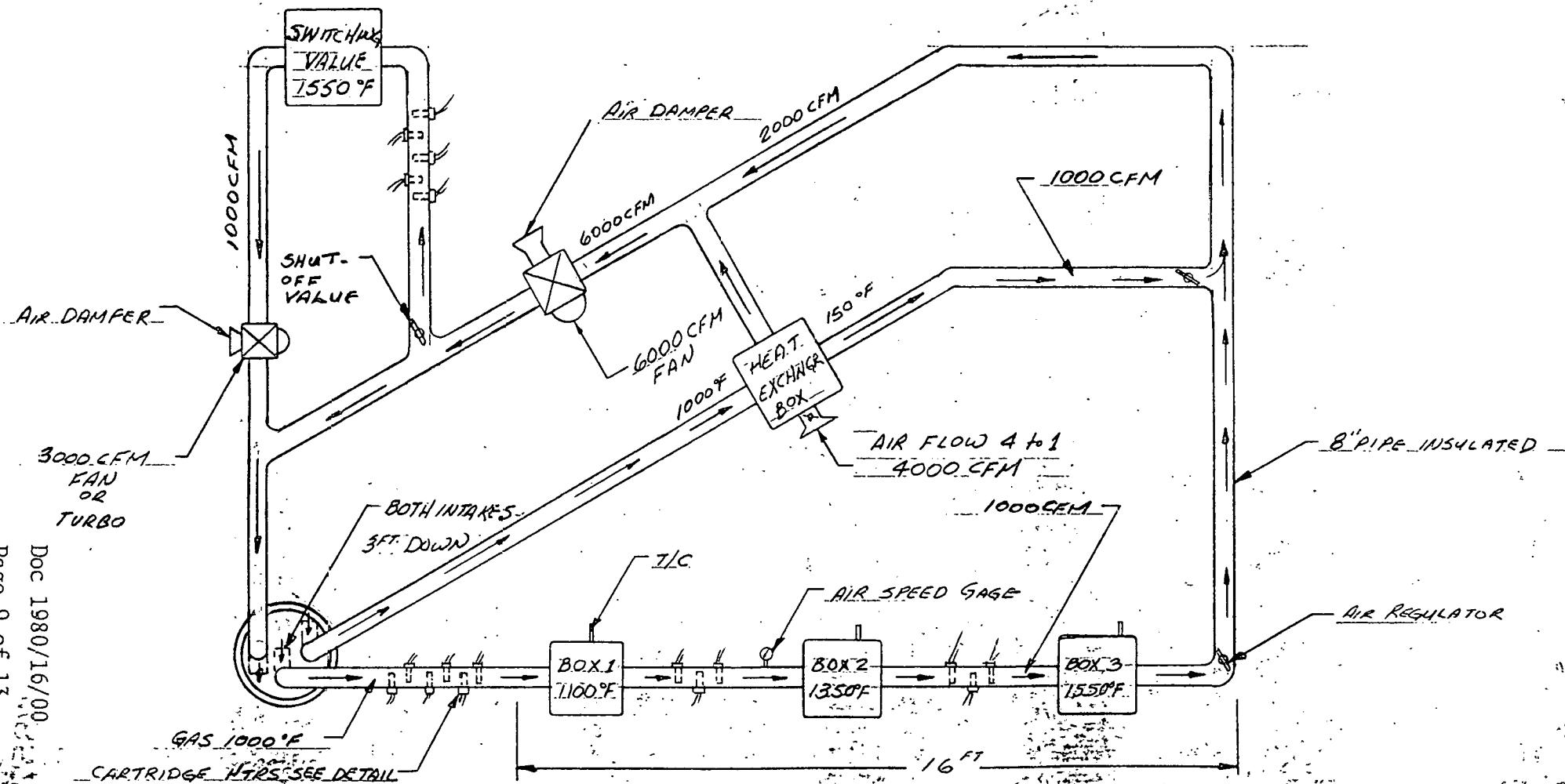
FIGURE 4.2 DETAIL OF CARTRIDGE HEATERS
