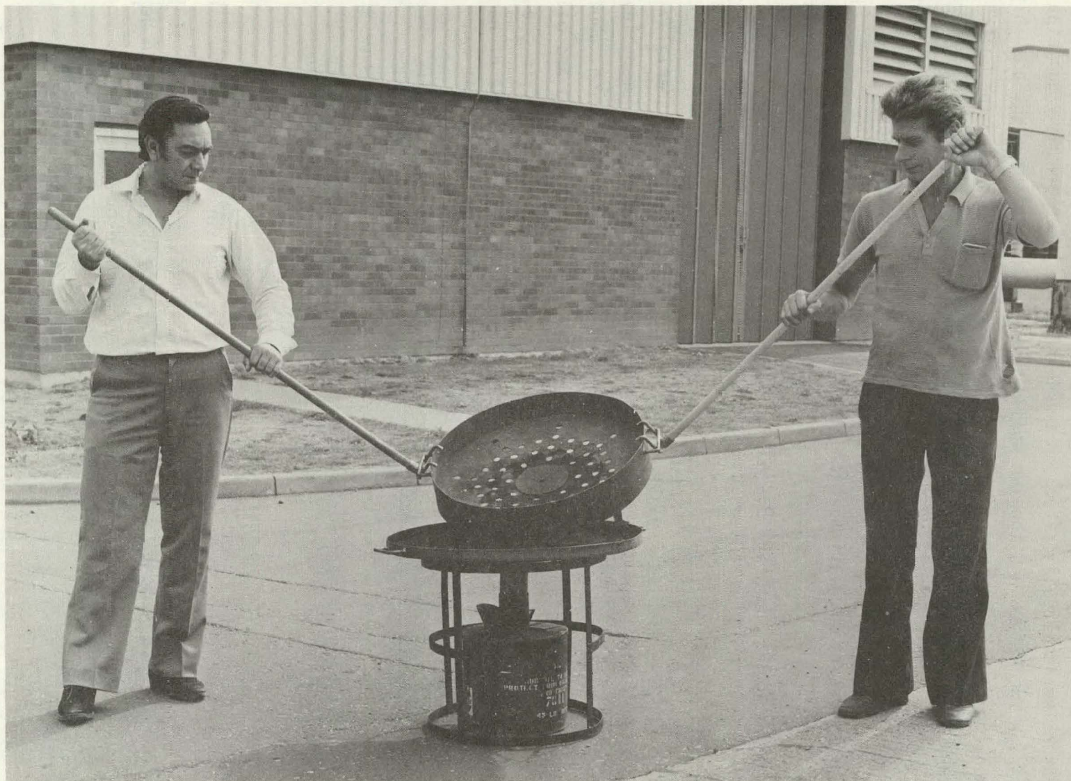
FIGURE 4.19. Portable Tar Ball Beach Incinerator Showing Size and Handling Source: Warren Springs Laboratory, Stevenage, England
