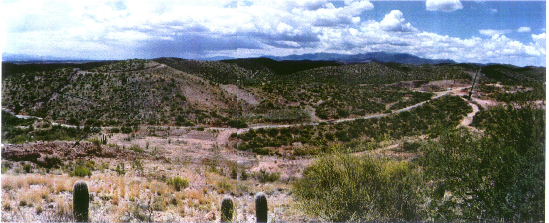
Figure 23: San Manuel site, AZ. Note the pronounced ground failures over the large cave area.
