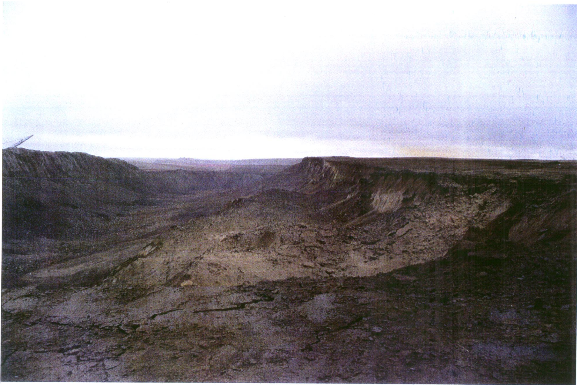
Figure 35: Black Thunder site, WY. Ground broken and thrown after a 1,600-ton ANFO cast shot.
