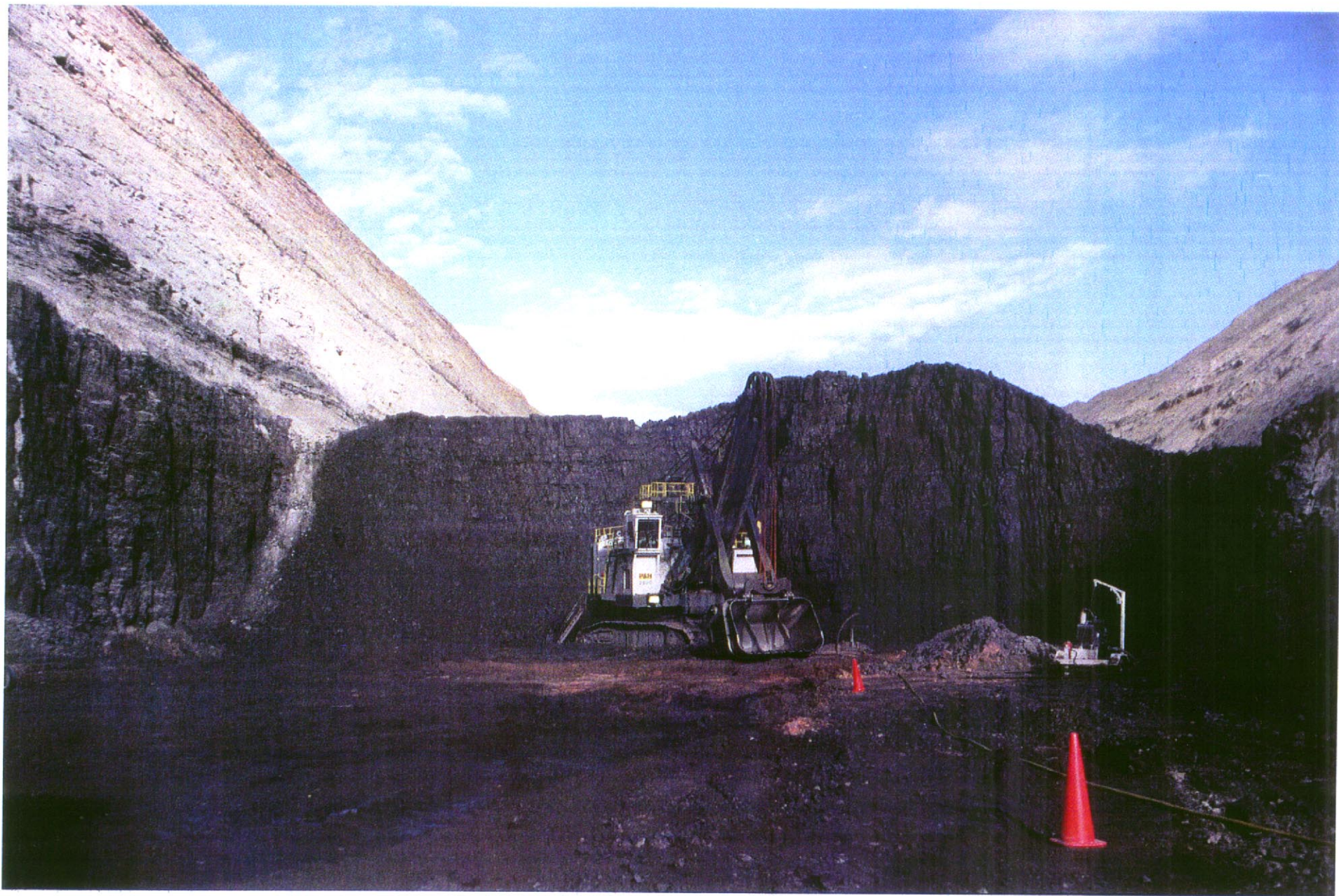
Figure 34: Black Thunder site, WY. 21-m thick coal seam.
