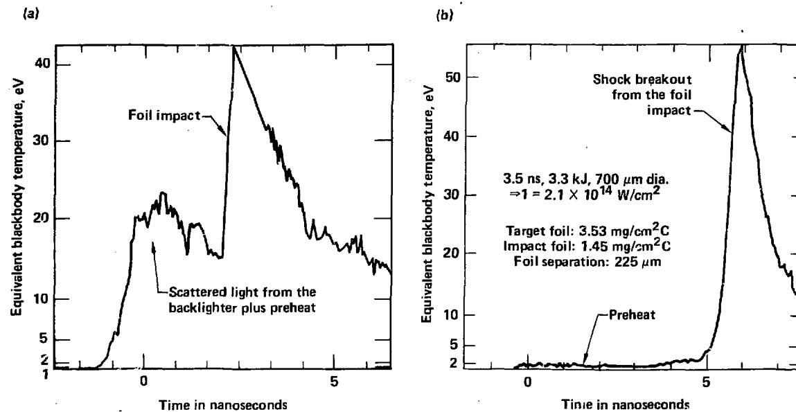
FIG. 4. (a) Time history of emission from rear of impact foil. Conditions as described in text.
