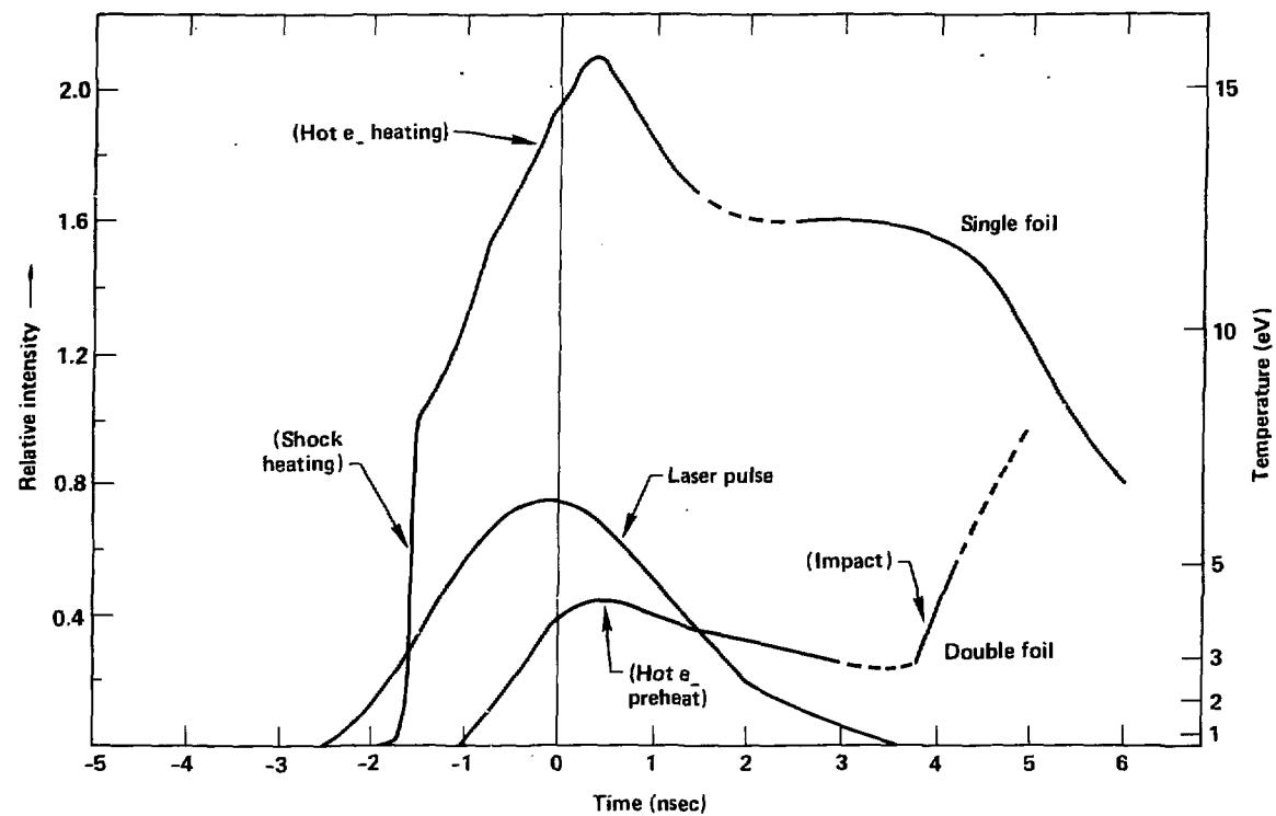
FIG. 2. Time history of emission from the rear of a single and double foil.
