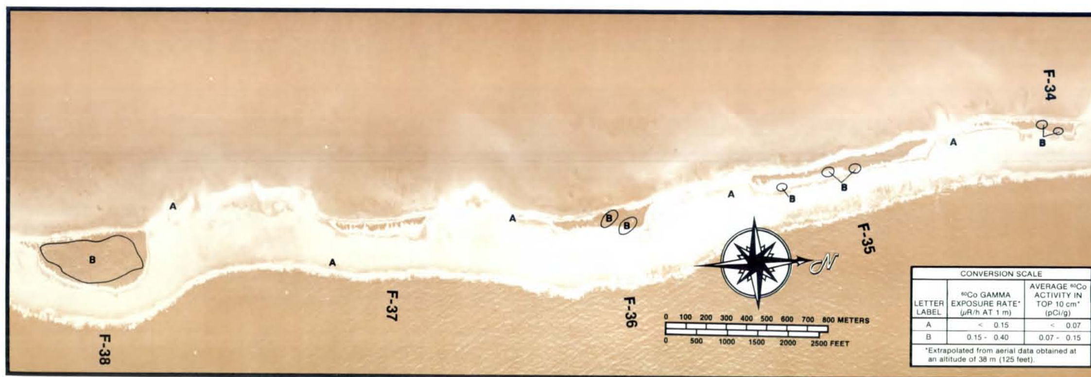
Figure D-37. COBALT 60 EXPOSURE RATE AND CONCENTRATION CONTOURS FOR ISLANDS F-34 TO F-38 AT RONGELAP ATOLL. (Photograph Frame Number 200)
