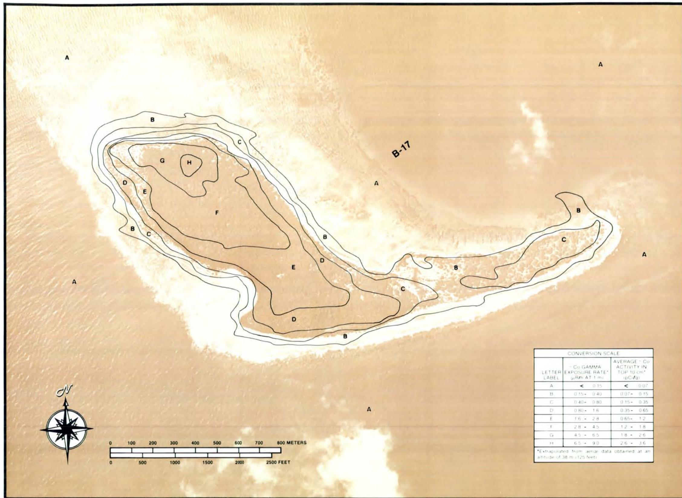
Figure D-172. COBALT 60 EXPOSURE RATE AND CONCENTRATION CONTOURS FOR ISLAND B-17 AT BIKINI ATOLL. (Photograph Frame Number 34)
