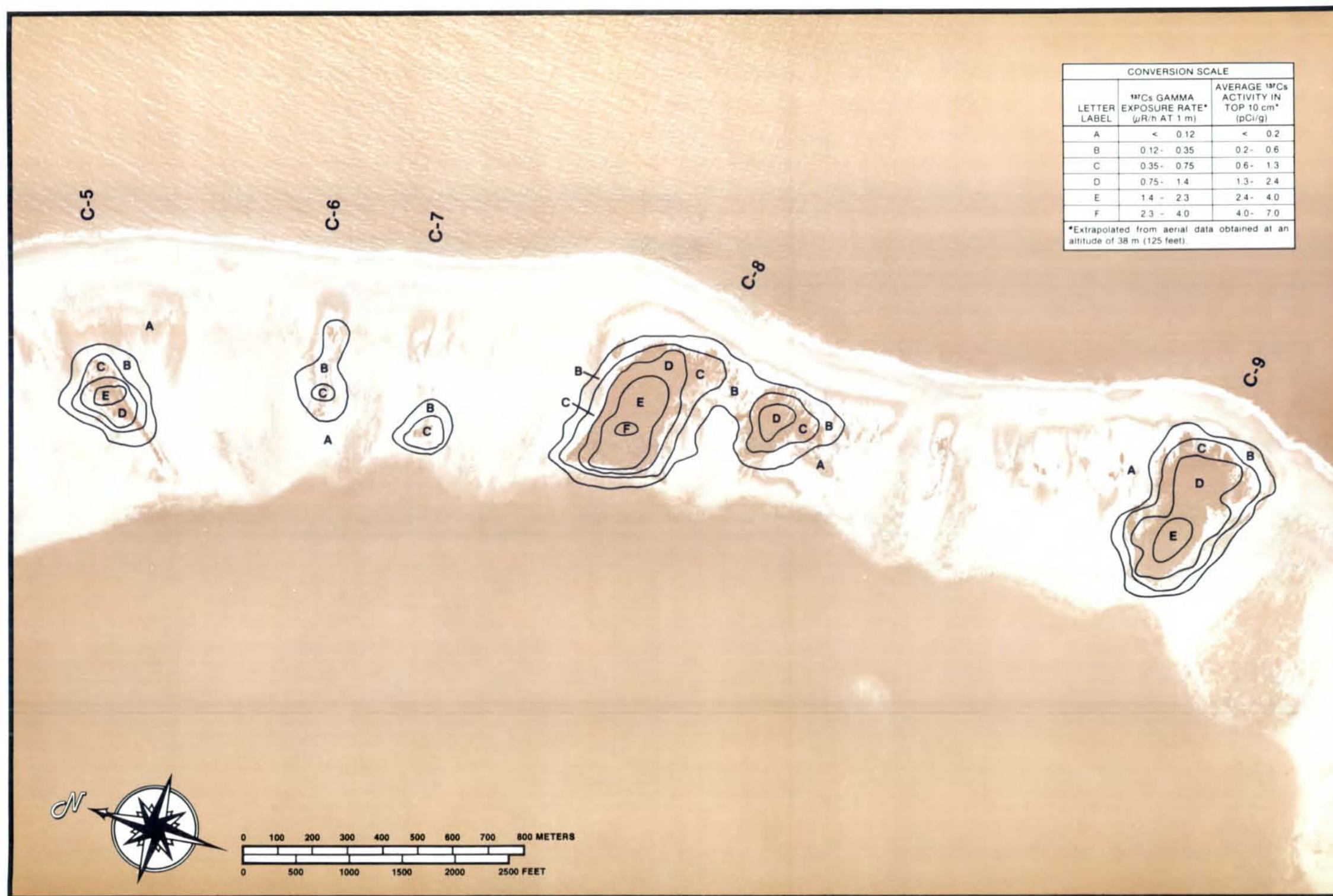
Figure D-89. CESIUM 137 EXPOSURE RATE AND CONCENTRATION CONTOURS FOR ISLANDS C-5 TO C-9 AT AILINGINAE ATOLL. (Photograph Frame Number 14)
