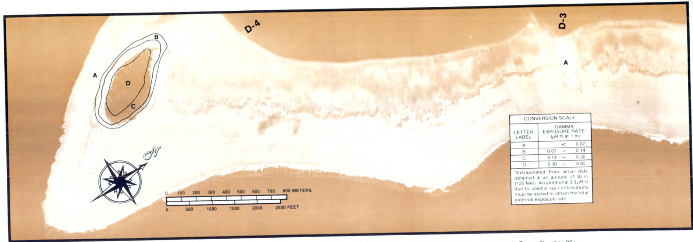
Figure D-65. TOTAL TERRESTRIAL EXPOSURE RATE CONTOURS FOR ISLANDS D-3 TO D-4 AT BIKAR ATOLL. (Photograph Frame Number 99)
