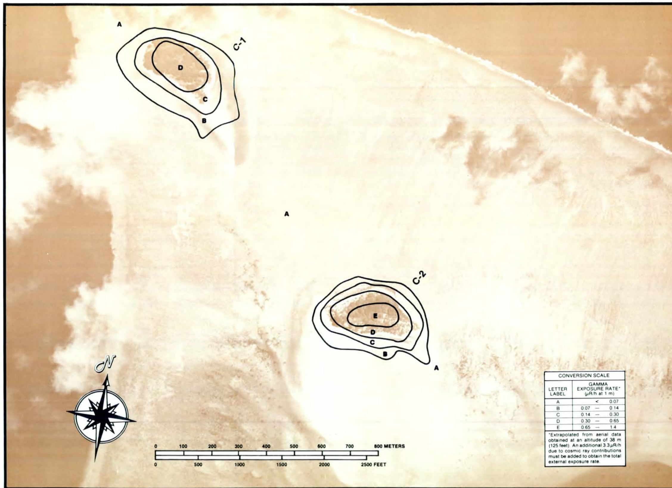
Figure D-84. TOTAL TERRESTRIAL EXPOSURE RATE CONTOURS FOR ISLANDS C-1 TO C-2 AT AILINGINAE ATOLL. (Photograph Frame Number 24)
