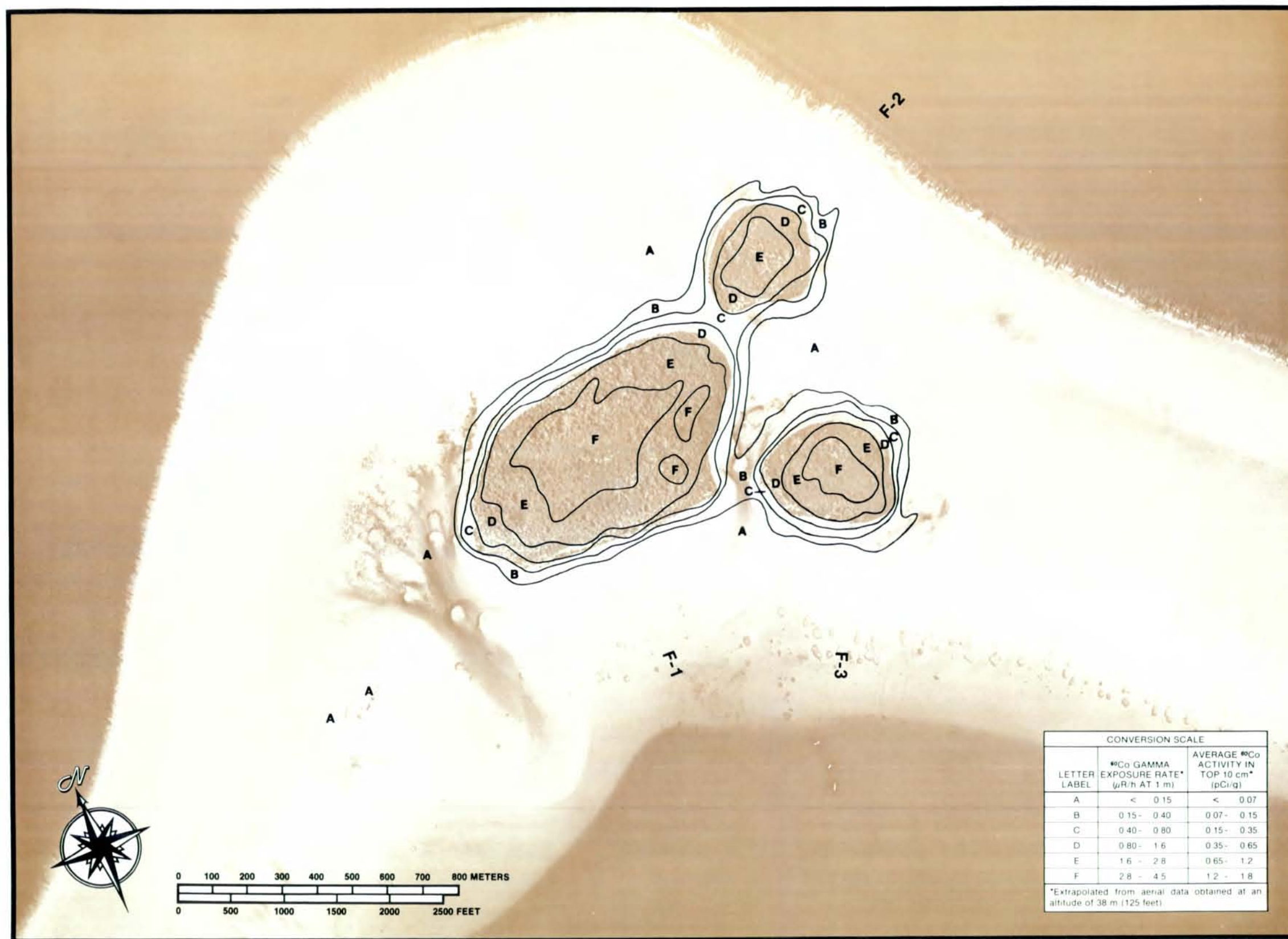
Figure D-4. COBALT 60 EXPOSURE RATE AND CONCENTRATION CONTOURS FOR ISLANDS F-1 TO F-3 AT RONGELAP ATOLL. (Photograph Frame Number 167)
