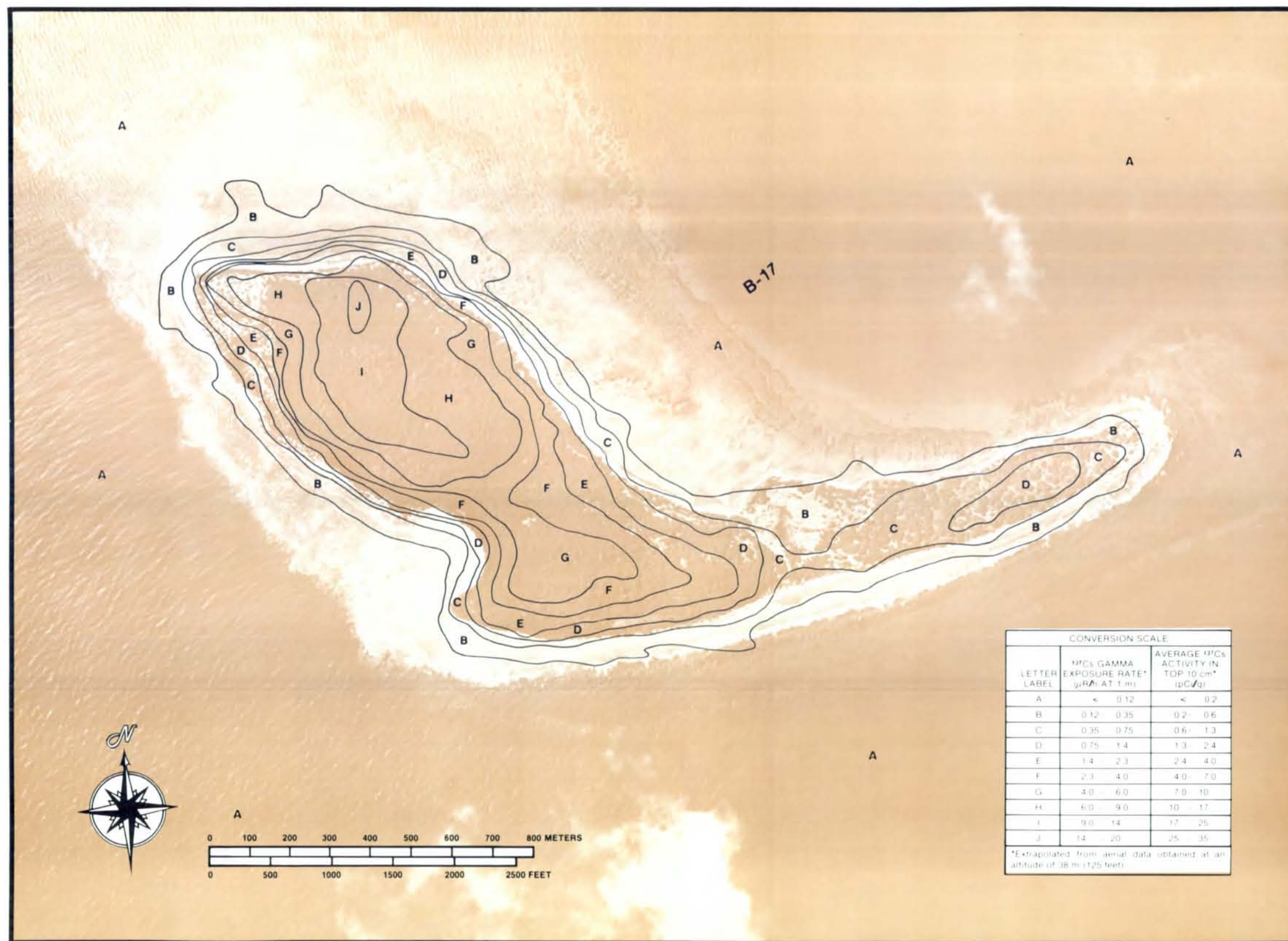
Figure D-171. CESIUM 137 EXPOSURE RATE AND CONCENTRATION CONTOURS FOR ISLAND B-17 AT BIKINI ATOLL. (Photograph Frame Number 34)
