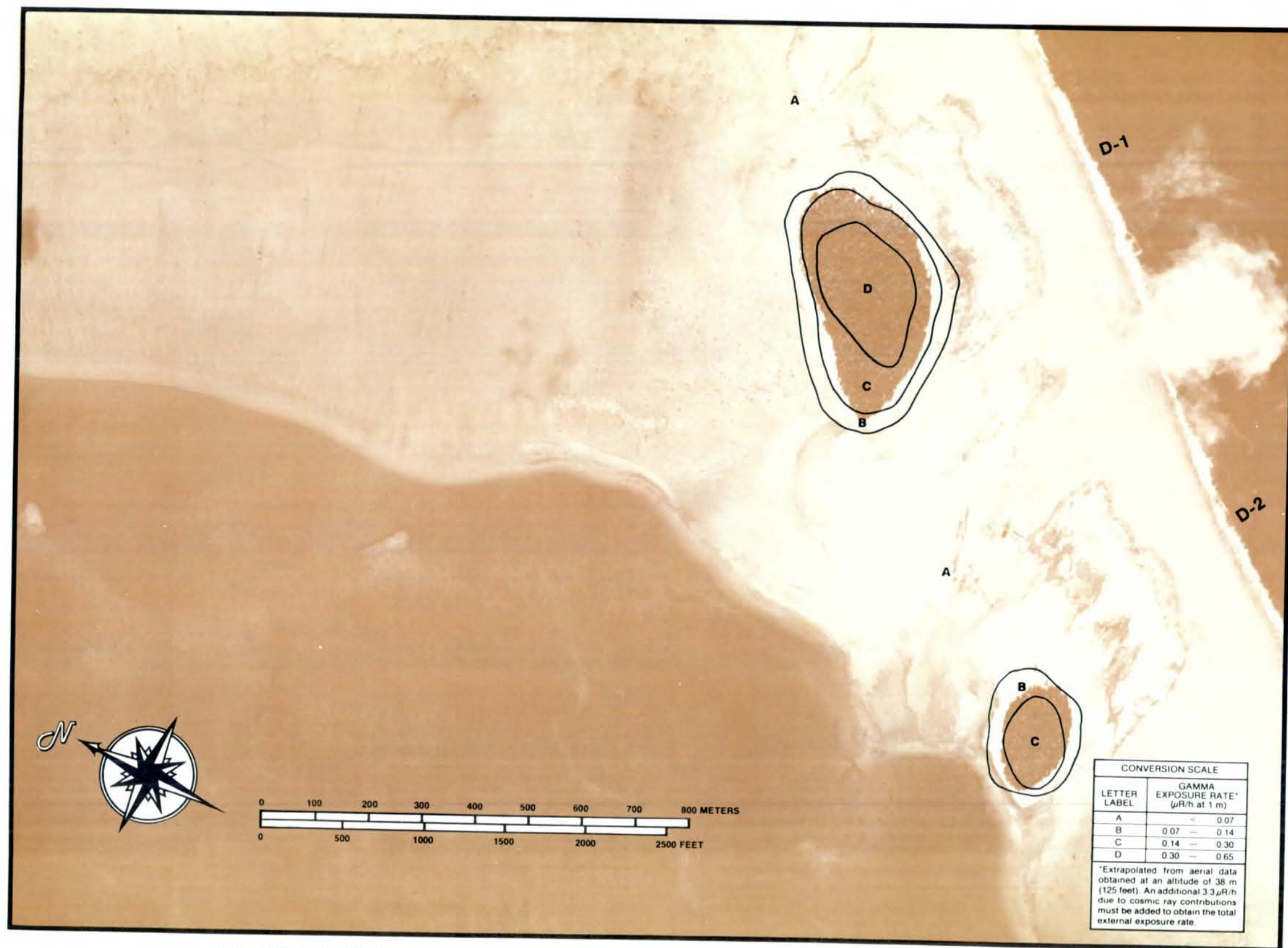
Figure D-64. TOTAL TERRESTRIAL EXPOSURE RATE CONTOURS FOR ISLANDS D-1 TO D-2 AT BIKAR ATOLL. (Photograph Frame Number 145)
