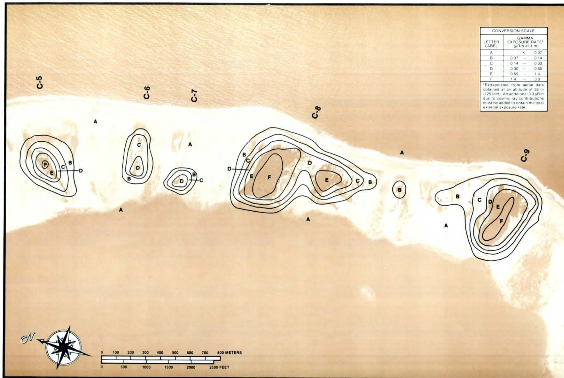
Figure D-88. TOTAL TERRESTRIAL EXPOSURE RATE CONTOURS FOR ISLANDS C-5 TO C-9 AT AILINGINAE ATOLL. (Photograph Frame Number 14)
