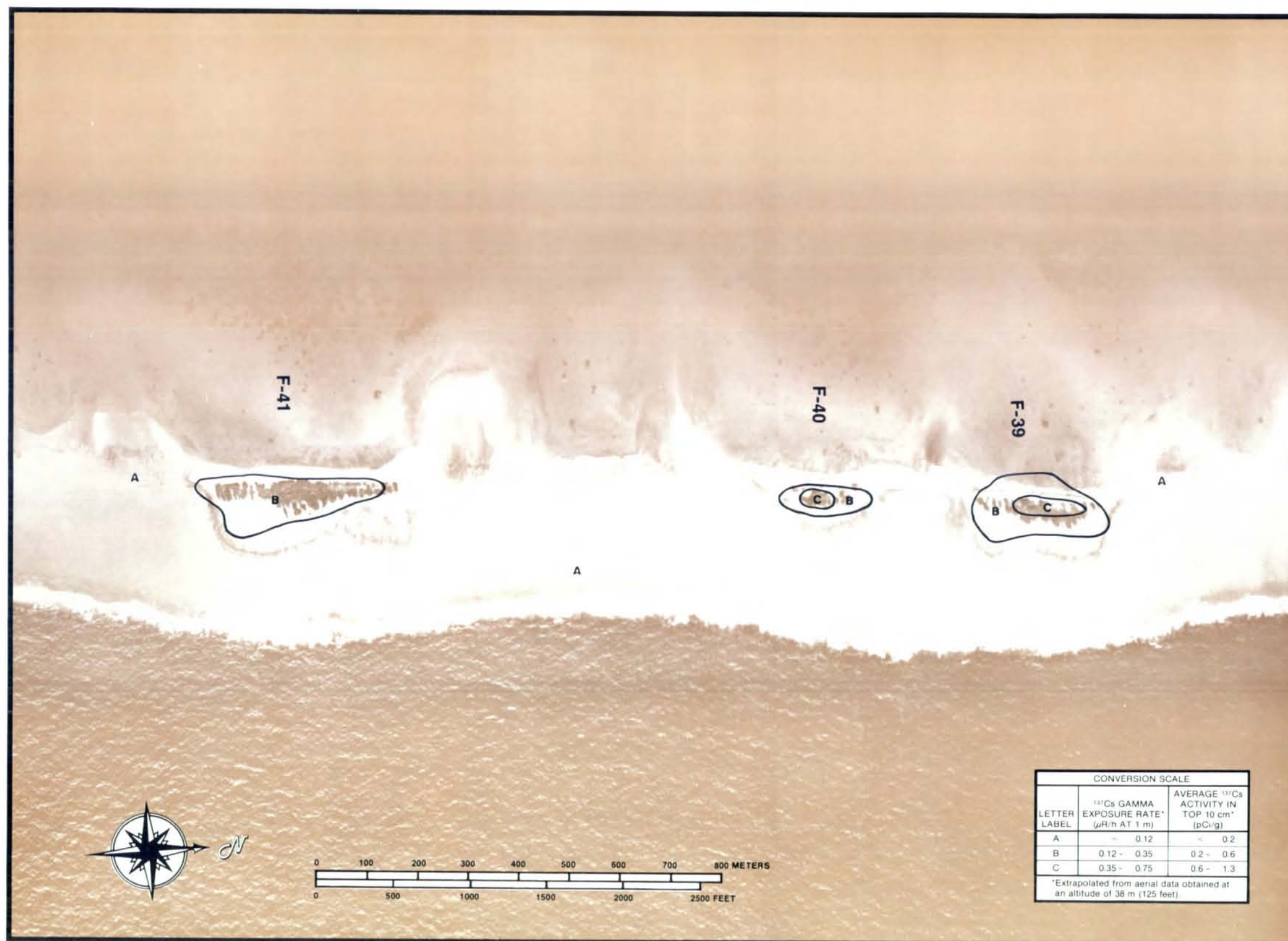
Figure D-39. CESIUM 137 EXPOSURE RATE AND CONCENTRATION CONTOURS FOR ISLANDS F-39 TO F-41 AT RONGELAP ATOLL. (Photograph Frame Number 196)
