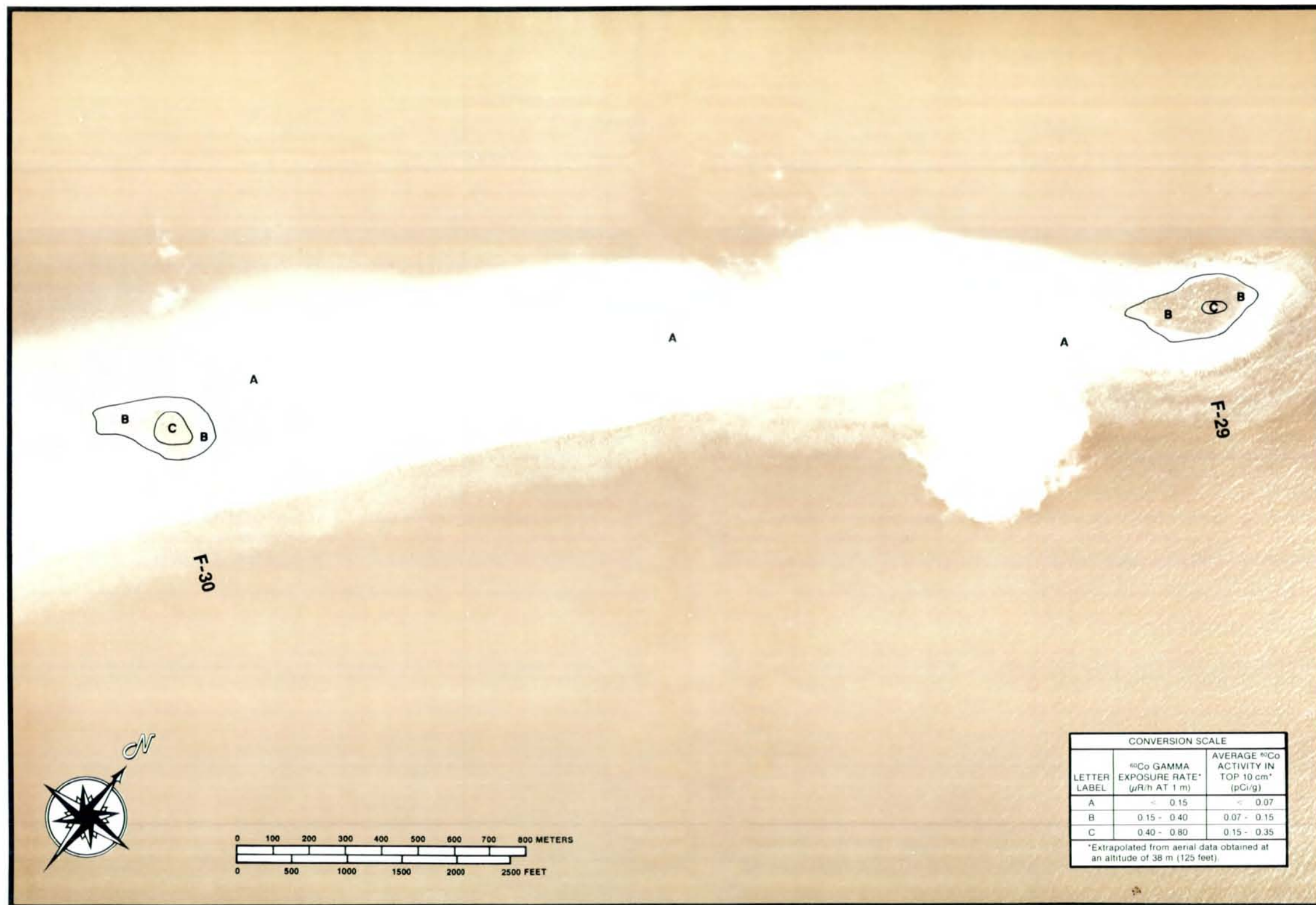
Figure D-31. COBALT 60 EXPOSURE RATE AND CONCENTRATION CONTOURS FOR ISLANDS F-29 TO F-30 AT RONGELAP ATOLL. (Photograph Frame Number 172)
