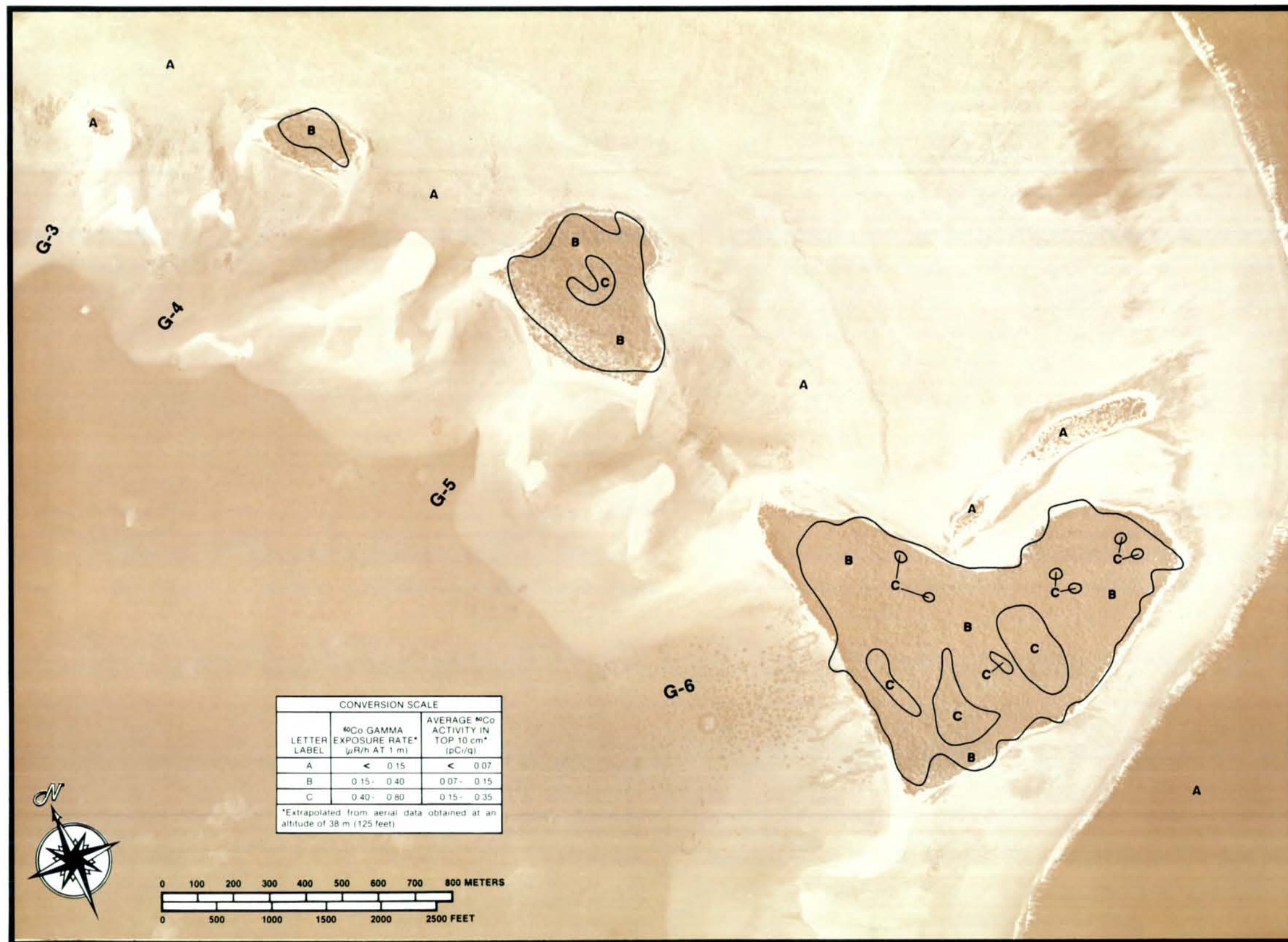
Figure D-73. COBALT-60 EXPOSURE RATE AND CONCENTRATION CONTOURS FOR ISLANDS G-3 TO G-6 AT RONGERIK ATOLL. (Photograph Frame Number 70)
