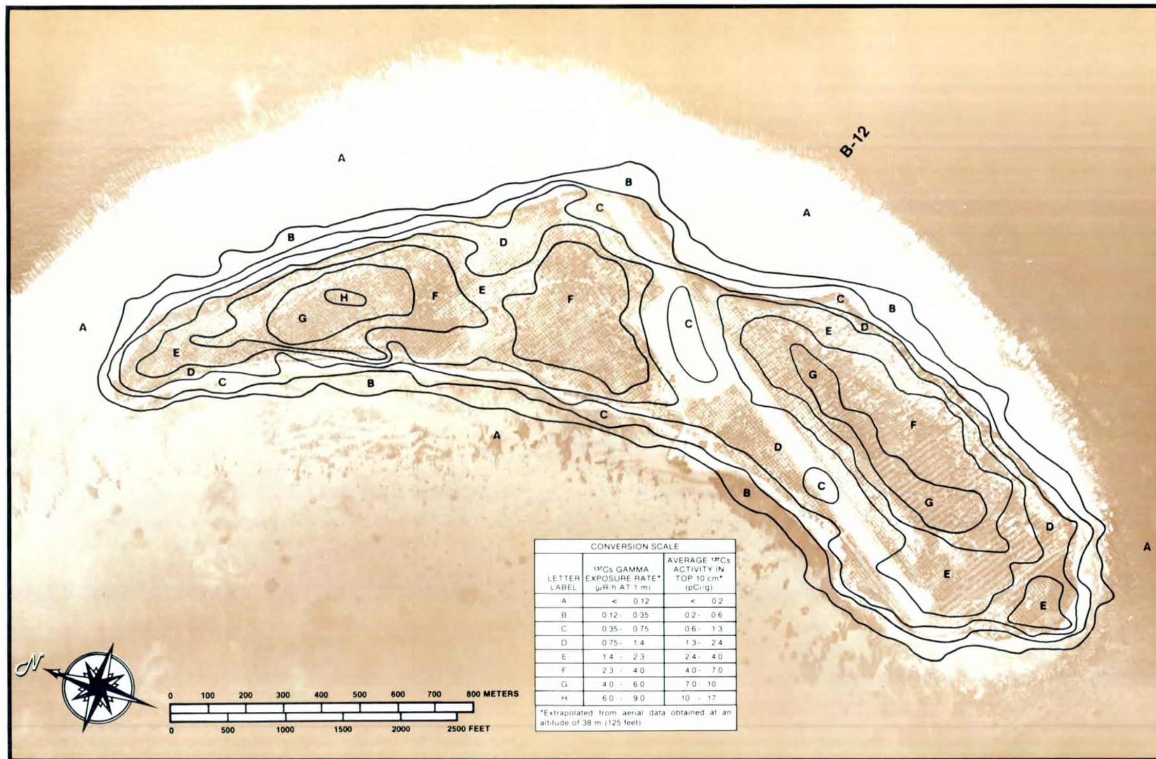
Figure D-165. CESIUM 137 EXPOSURE RATE AND CONCENTRATION CONTOURS FOR ISLAND B-12 AT BIKINI ATOLL. (Photograph Frame Number 200)
