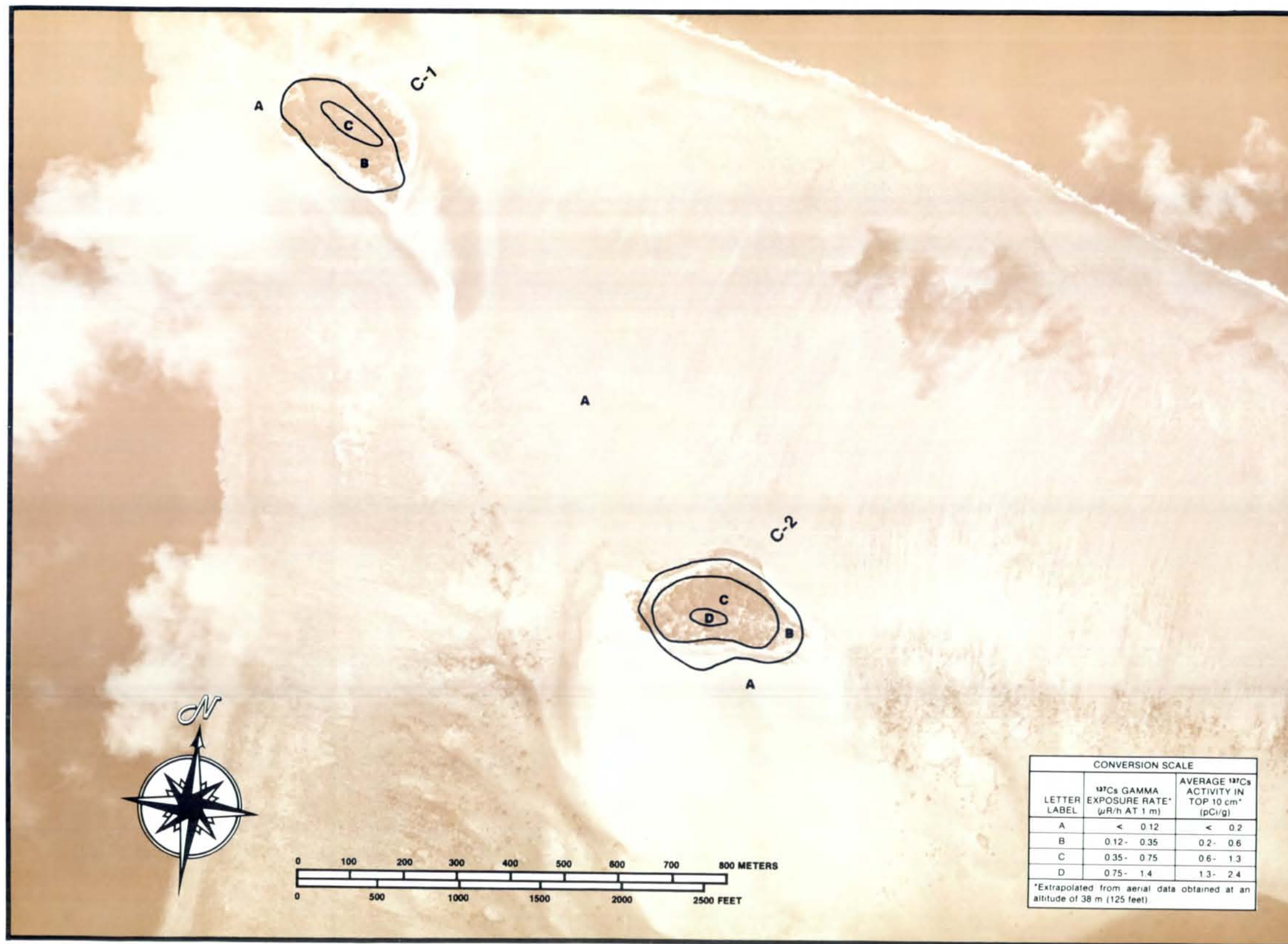
Figure D-85. CESIUM 137 EXPOSURE RATE AND CONCENTRATION CONTOURS FOR ISLANDS C-1 TO C-2 AT AILINGINAE ATOLL. (Photograph Frame Number 24)
