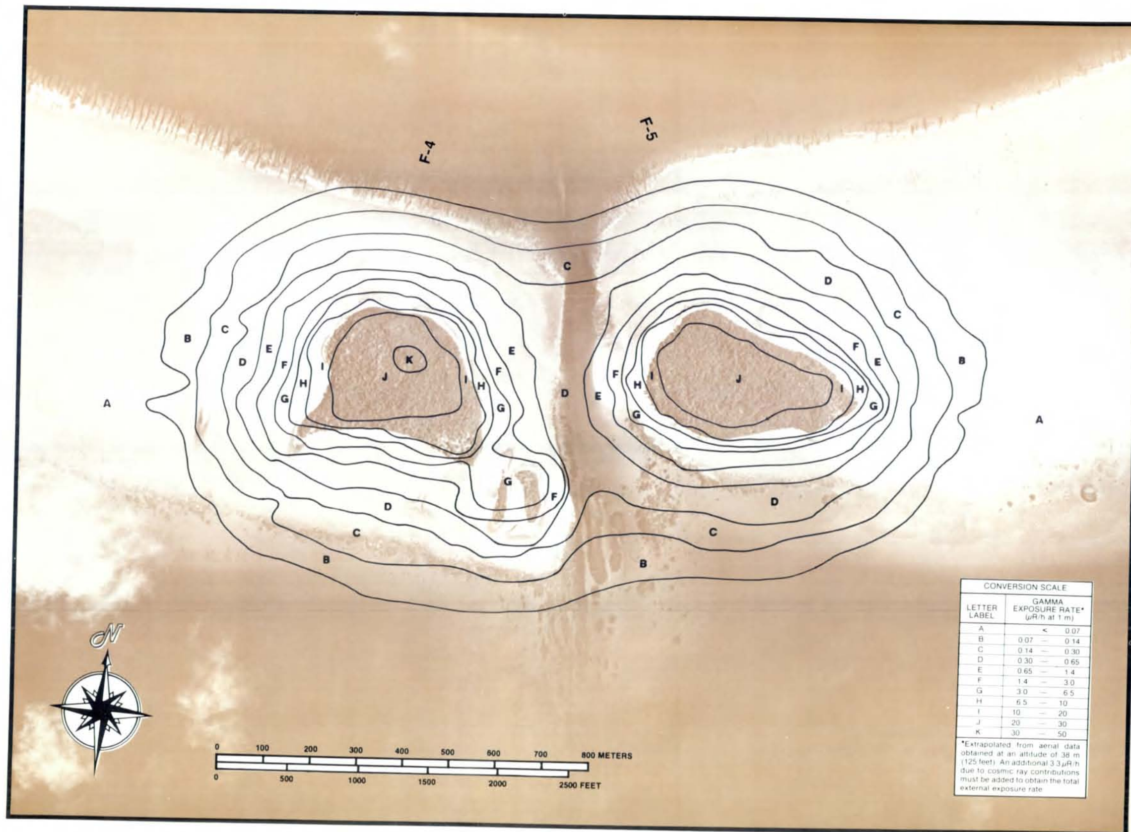
Figure D-5. TOTAL TERRESTRIAL EXPOSURE RATE CONTOURS FOR ISLANDS F-4 TO F-5 AT RONGELAP ATOLL. (Photograph Frame Number 159)
