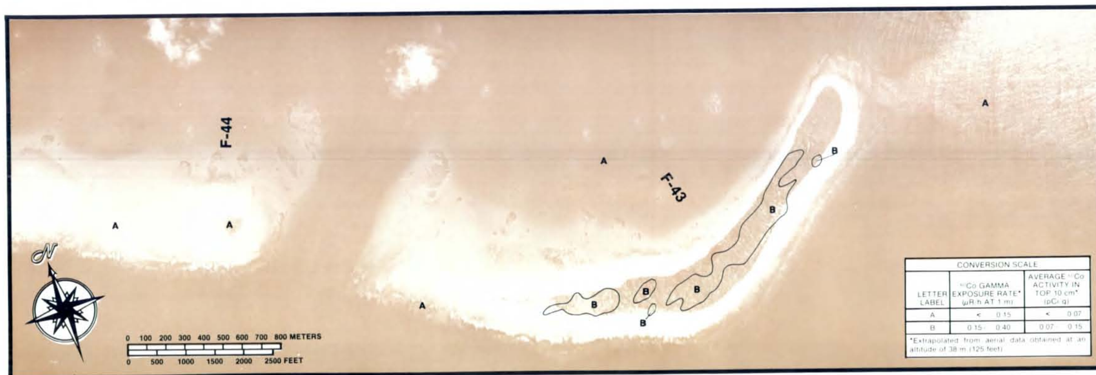
Figure D-46. COBALT 60 EXPOSURE RATE AND CONCENTRATION CONTOURS FOR ISLANDS F-43 TO F-44 AT RONGELAP ATOLL. (Photograph Frame Number 72)
