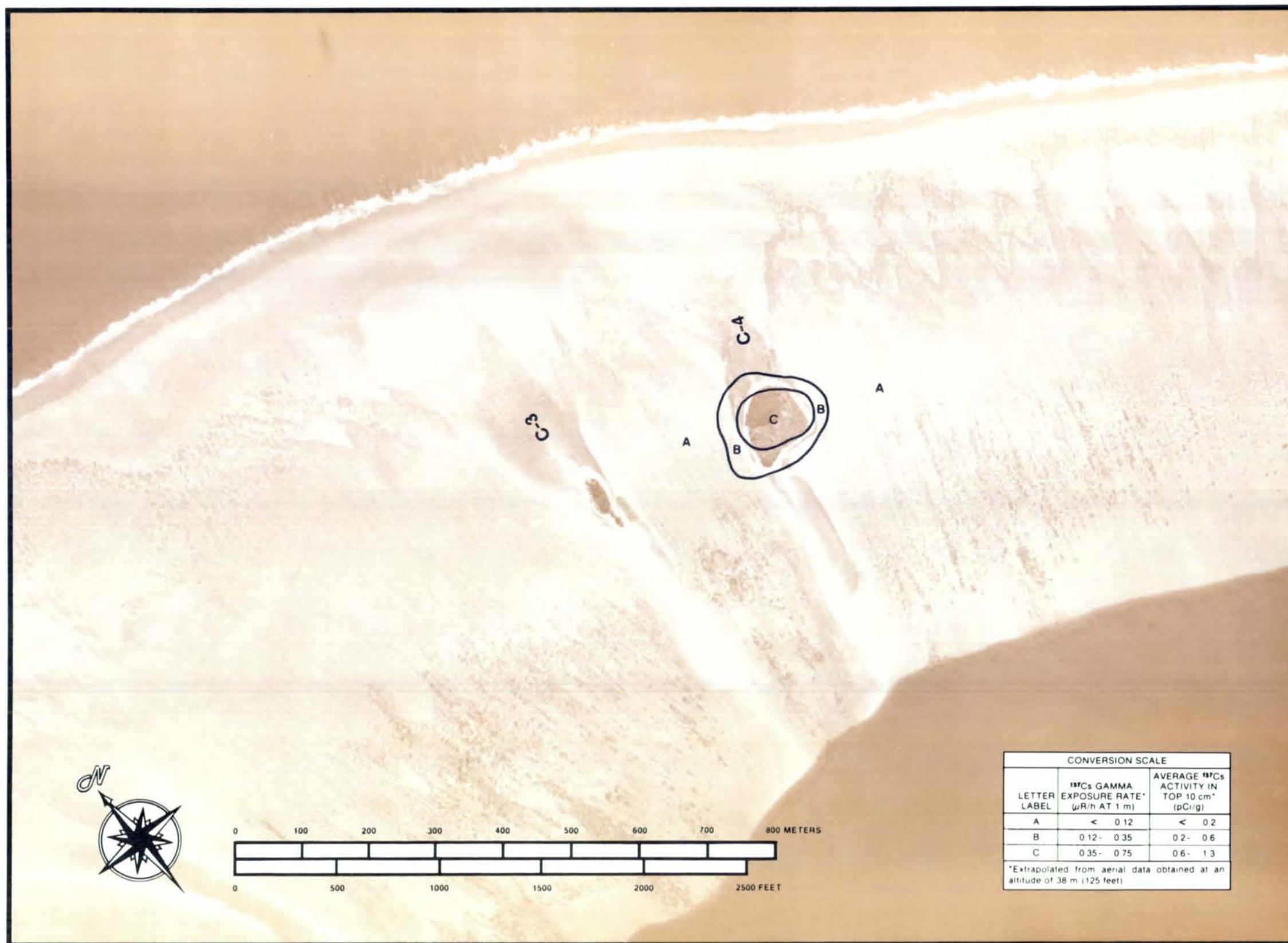
Figure D-87. CESIUM 137 EXPOSURE RATE AND CONCENTRATION CONTOURS FOR ISLANDS C-3 TO C-4 AT AILINGINAE ATOLL. (Photograph Frame Number 17)
