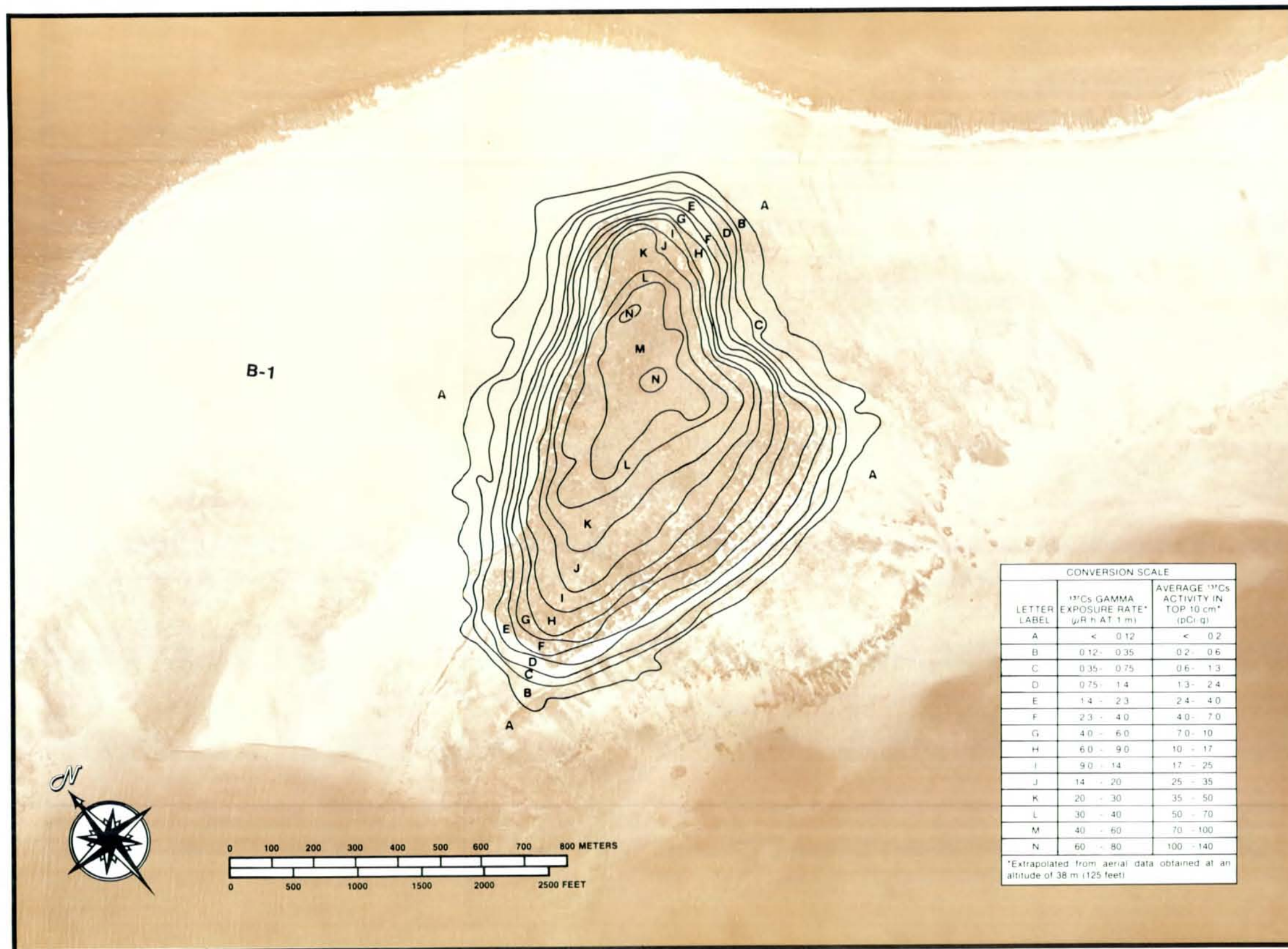
Figure D-153. CESIUM 137 EXPOSURE RATE AND CONCENTRATION CONTOURS FOR ISLAND B-1 AT BIKINI ATOLL. (Photograph Frame Number 177)
