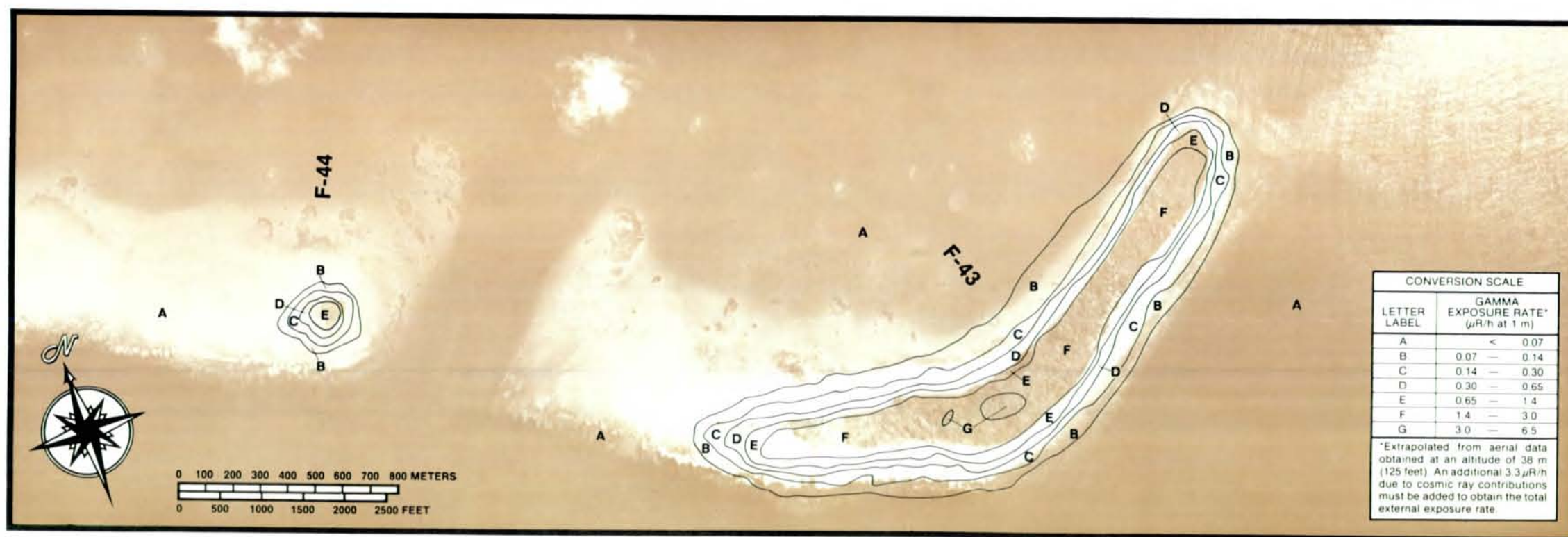
Figure D-44. TOTAL TERRESTRIAL EXPOSURE RATE CONTOURS FOR ISLANDS F-43 TO F-44 AT RONGELAP ATOLL. (Photograph Frame Number 72)
