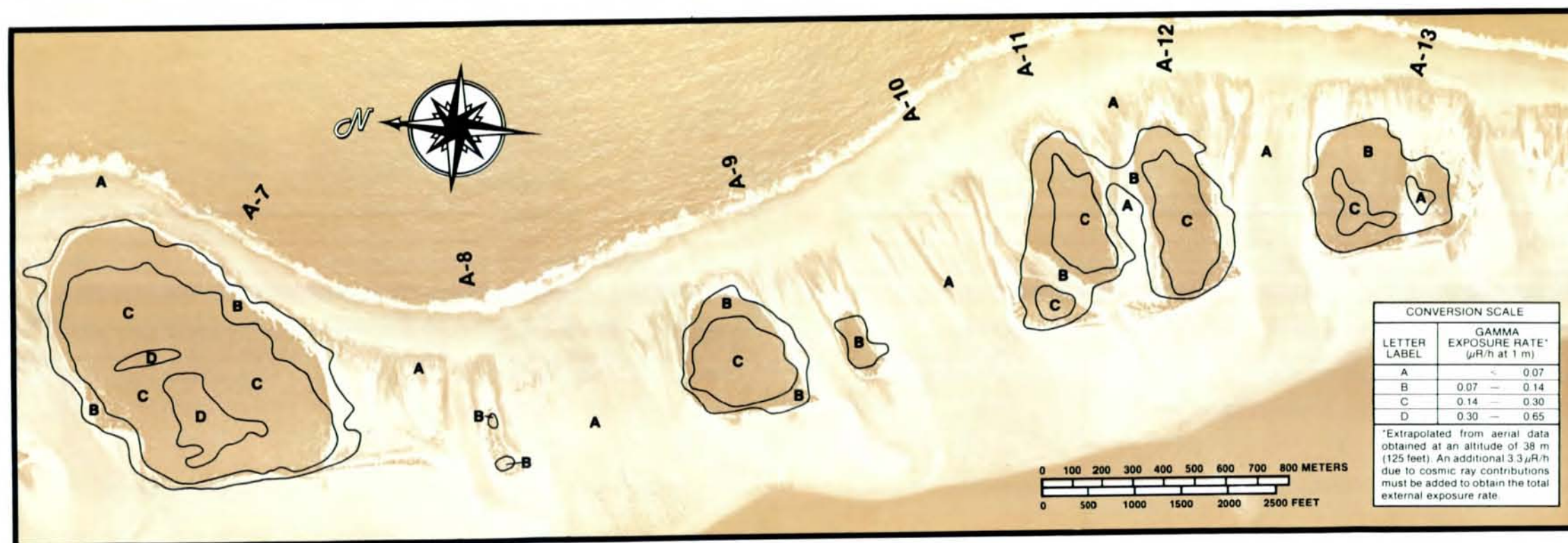
Figure D-123. TOTAL TERRESTRIAL EXPOSURE RATE CONTOURS FOR ISLANDS A-7 TO A-13 AT AILUK ATOLL (Photograph Frame Number 122)
