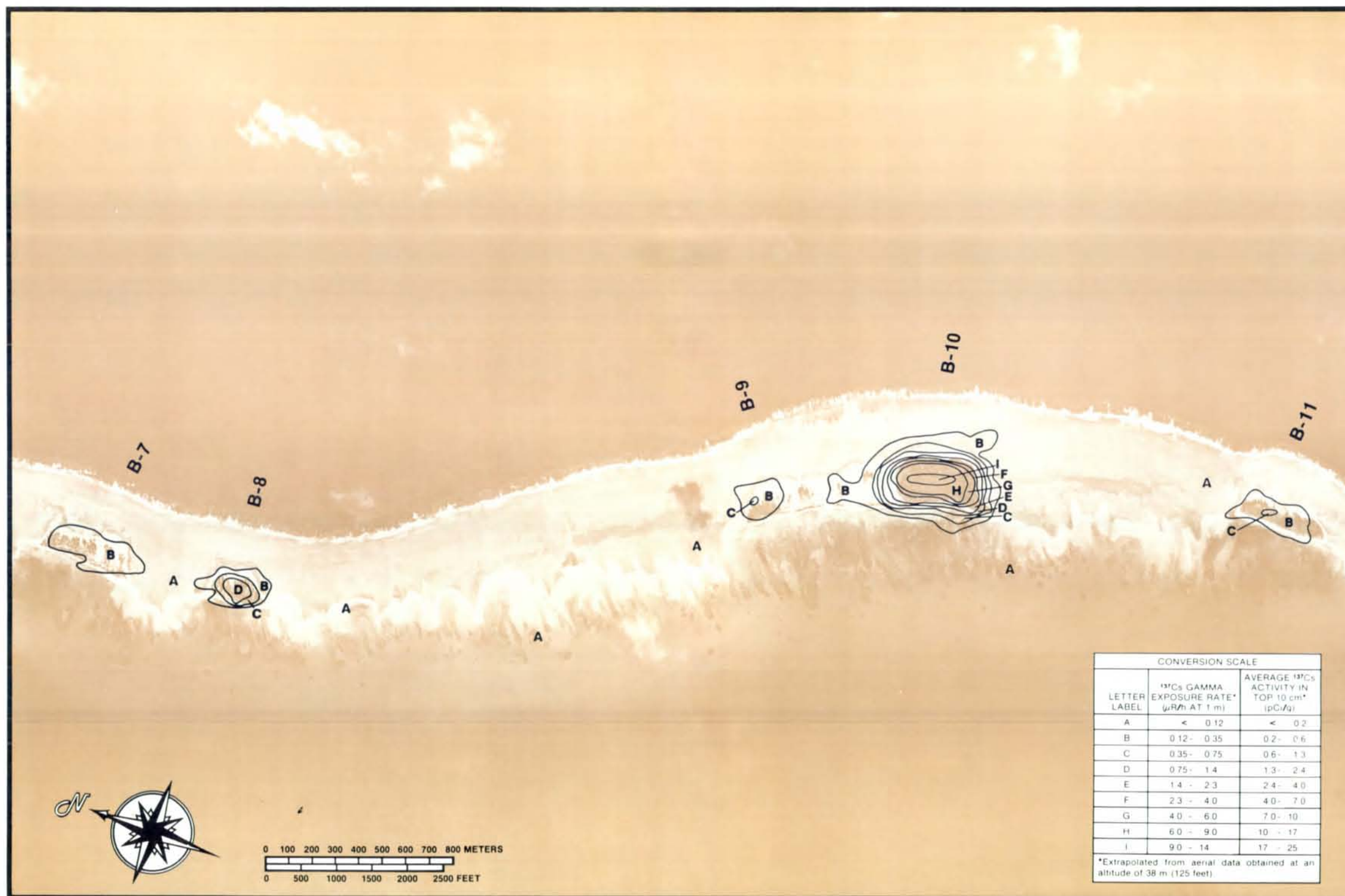
Figure D-162. CESIUM 137 EXPOSURE RATE AND CONCENTRATION CONTOURS FOR ISLANDS B-7 TO B-11 AT BIKINI ATOLL. (Photograph Frame Number 7)
