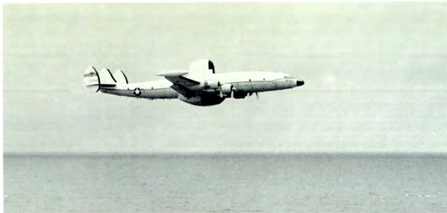
Figure 1. U.S. NAVY EC-121 AIRCRAFT USED FOR THE AERIAL PHOTOGRAPHIC MISSIONS. Both aerial camera ports and the navigation sight were mounted in the fuselage forward of the engines.
