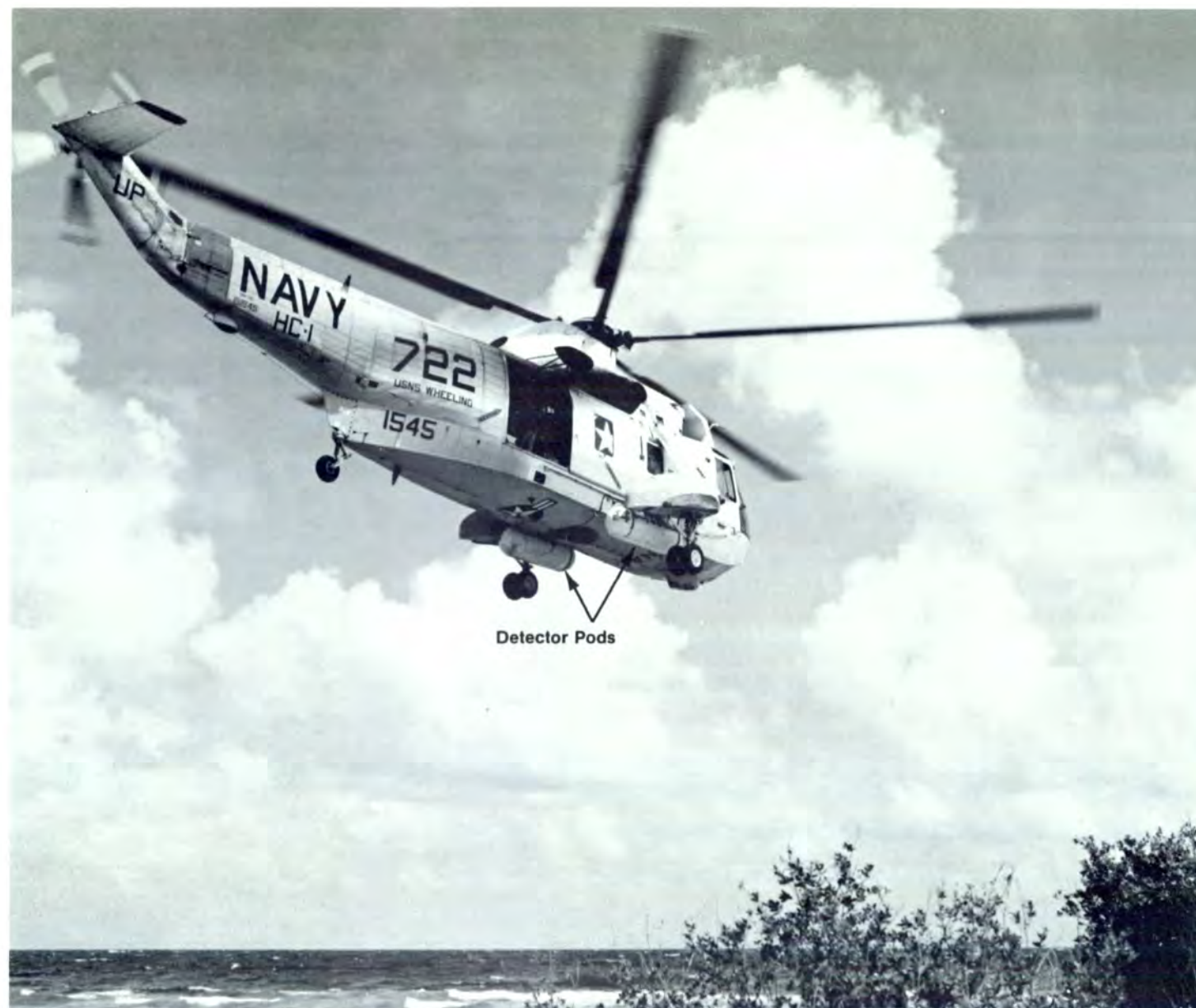
Figure 9. A NAVY SH-3G HELICOPTER WITH GAMMA RADIATION DETECTOR PODS ATTACHED
