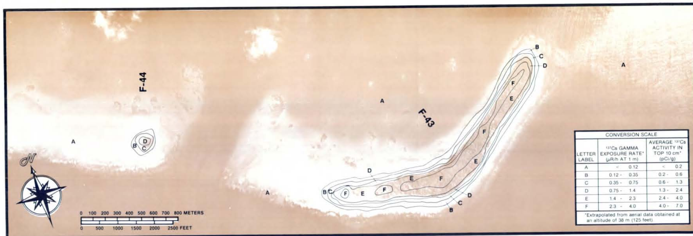
Figure D-45. CESIUM 137 EXPOSURE RATE AND CONCENTRATION CONTOURS FOR ISLANDS F-43 TO F-44 AT RONGELAP ATOLL. (Photograph Frame Number 72)
