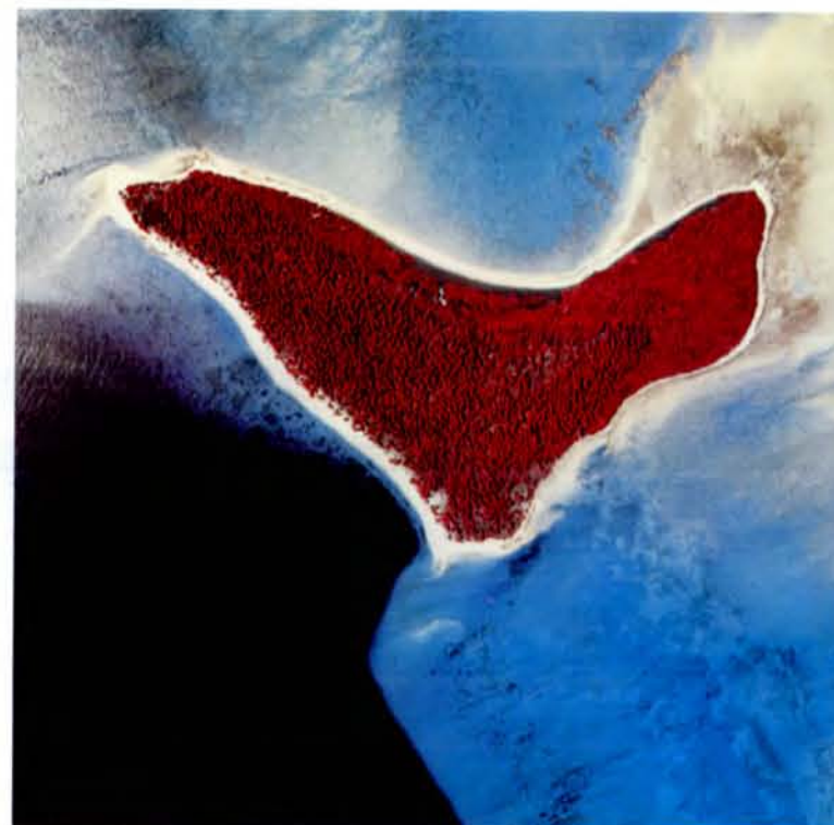
Infrared or "false" color photographic record of the wavelength region between 500 nm and 900 nm.
