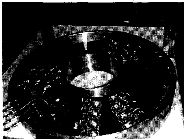
Fig. 3 Photograph of the high-voltage junction box including the AMPTEK boards.
