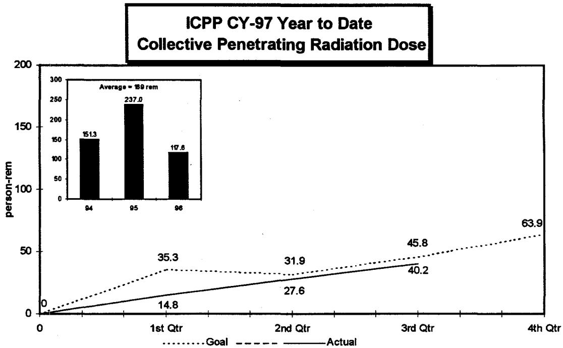
The ICPP collective penetrating occupational radiation exposure through the end of the third quarter was 40.155 person-rem. Decontamination and shielding on the Tank Farm, startup of NWCF, and some work being deferred or cancelled have contributed to an adjustment of the ICPP goal to 63.865 rem. The deferred work accounts for the dip in the goal line.
