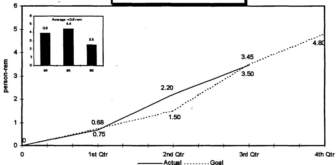
The collective penetrating occupational radiation exposure at CFA through the end of the third quarter is 3.454 person-rem. The major contributor has been Decontamination and Decommissioning (D&D) at ARA. The effort has resulted in significantly more scope than originally planned. Therefore the ALARA goal was reviewed and increased by 1.8 person-rem.
