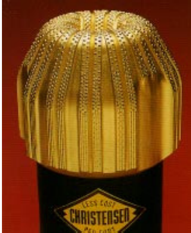
At its Elk Hills Naval Petroleum Reserve in California, the Department of Energy used a diamond drill bit similar to this to achieve a record-setting 1,058 hours of drilling operations without having to remove the bit. Diamond bits generally are run between 230 and 260 hours without a trip.
