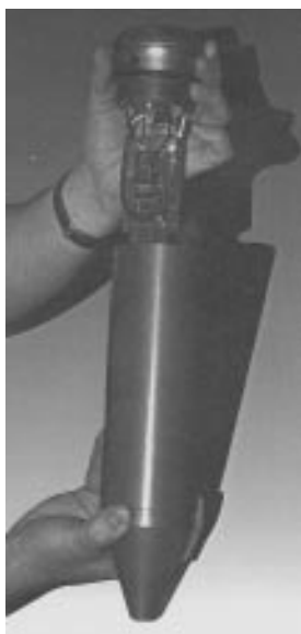
An Automatic Casing Swab
