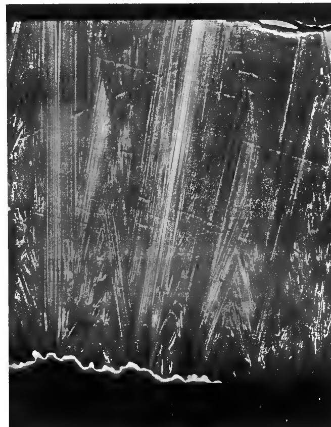
CROSS-SECTION OF SILICON RIBBON FROM SUBSTRATE USED 4 TIMES 320X
