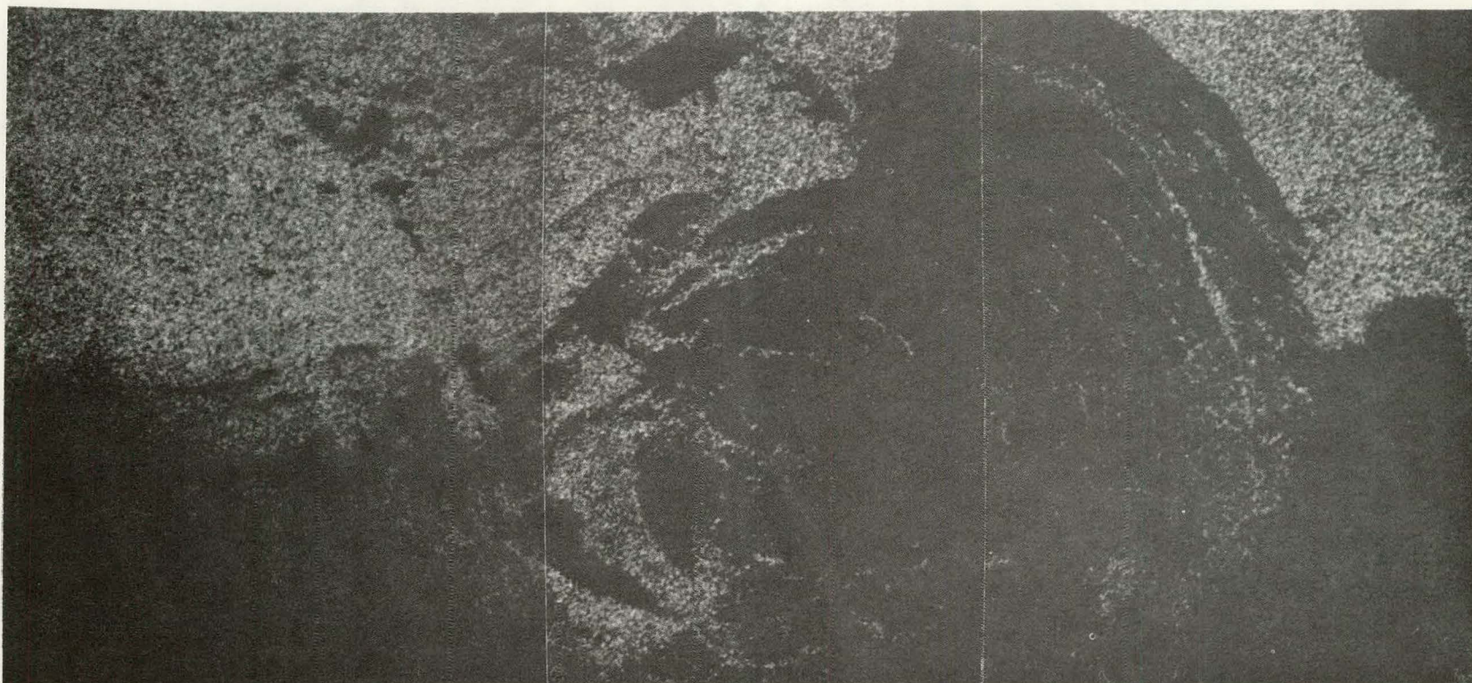
Figure 6. SCANNING ELECTRON MICROSCOPE ALUMINUM X-RAY MAP THAT VERIFIES THOSE AREAS WHICH ARE VOID OF ALUMINUM (THE DARK AREAS). (This Area is the same as that in Figure 5; ~ 70X)
