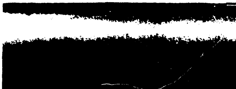
Cross section, x-contrast, scanning transmission electron micrograph from a silicon sample implanted at 80 keV with antimony. The light areas are due to enhanced electron scattering from the near-Gaussian antimony implantation distribution.
