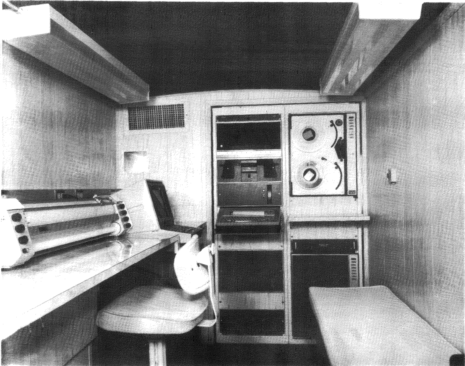
Figure 17. Interior of the mobile van which houses the Radiation and Environmental Data Analyzer and Computer (REDAC) system, used in analysis of the survey data.
