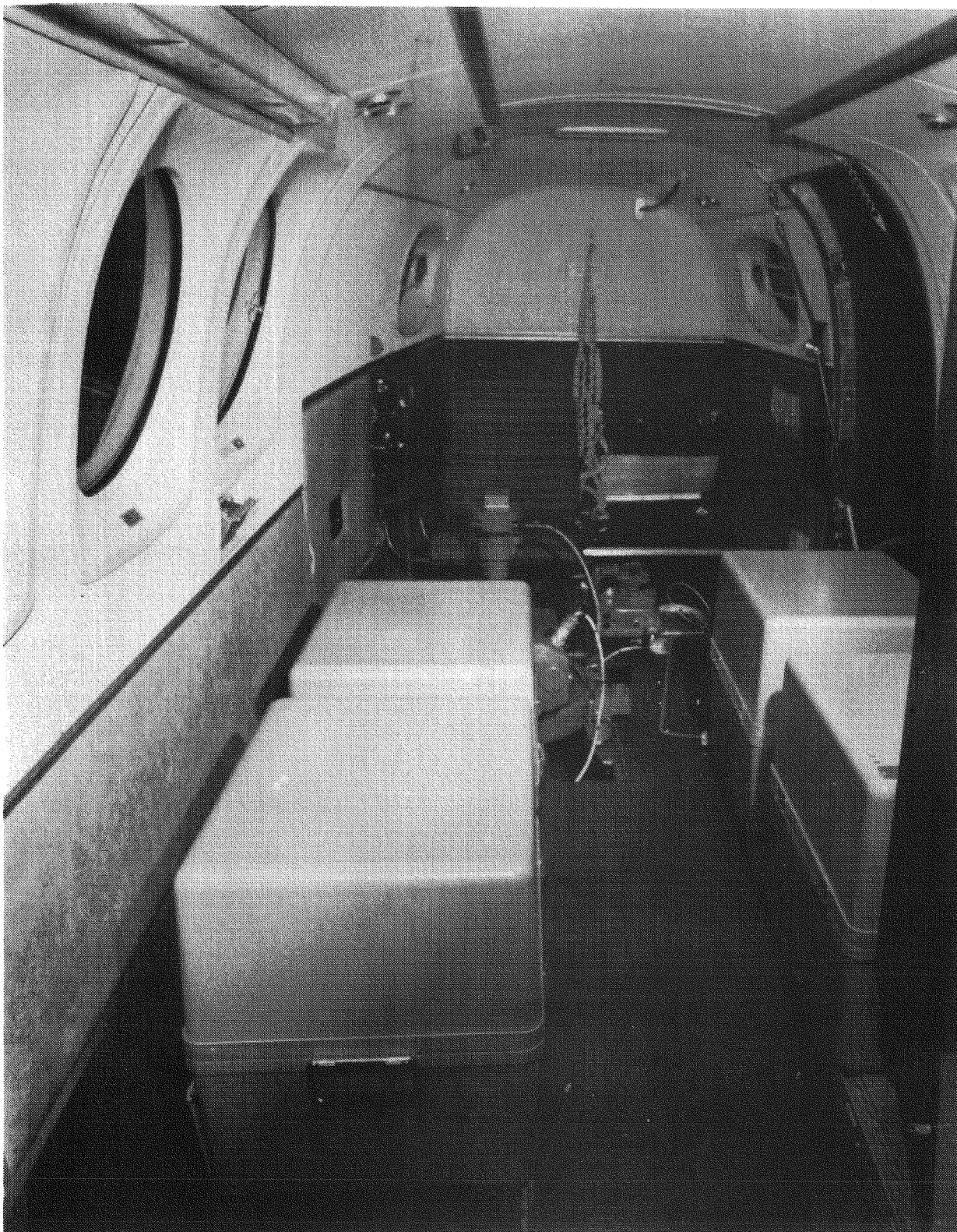
Figure 4. The four detector arrays mounted in the aft section of the ARMS aircraft.
