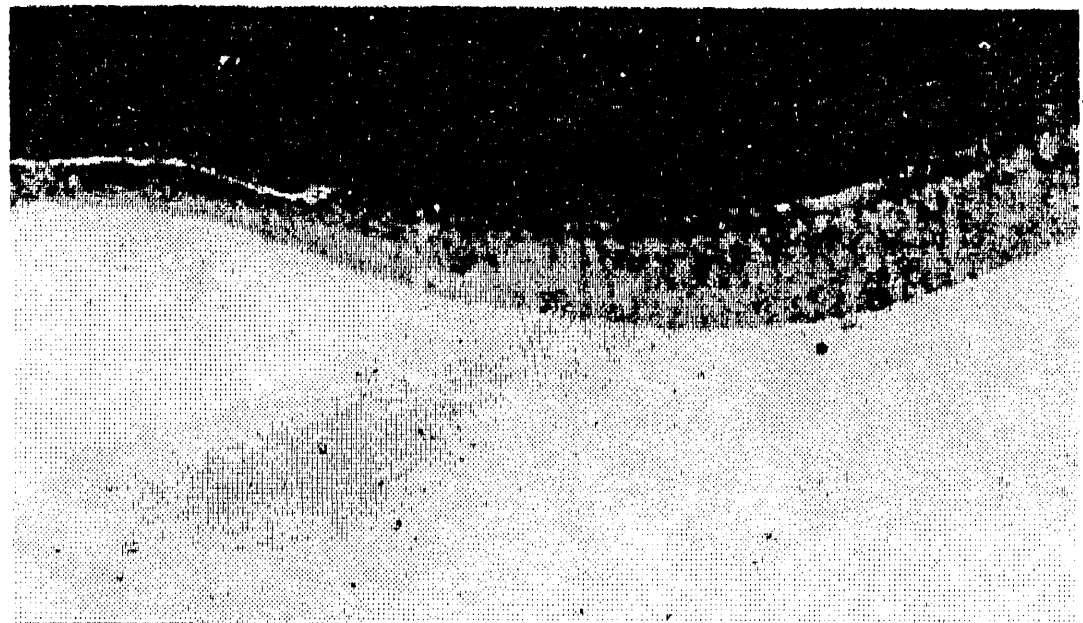
Figure 4.43 Corroded Surface of 72 Weld Wire Deposited on Incoloy 800 Base Metal Coated With 10 wt% Alkali Sulfates After Exposure for 800 Hours at 700°C to 0.25 vol% SO 2 . (Note thin layer of 800 on top of welded overlay.)
