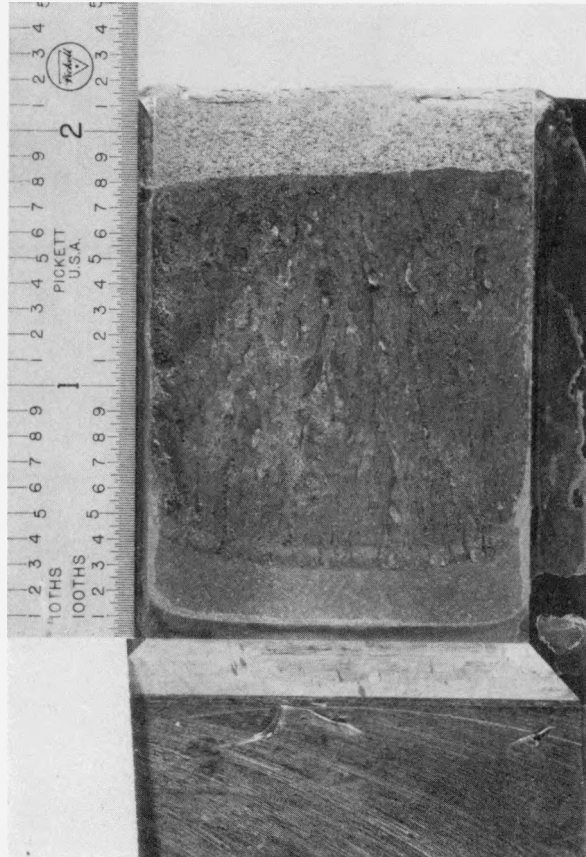
Fig. 3. Fracture surface of deeply side grooved 2T compact tension specimen 54H tested in 50 psig H_2S . This specimen exhibits little or no effect from plane-stress on either side of the crack front
