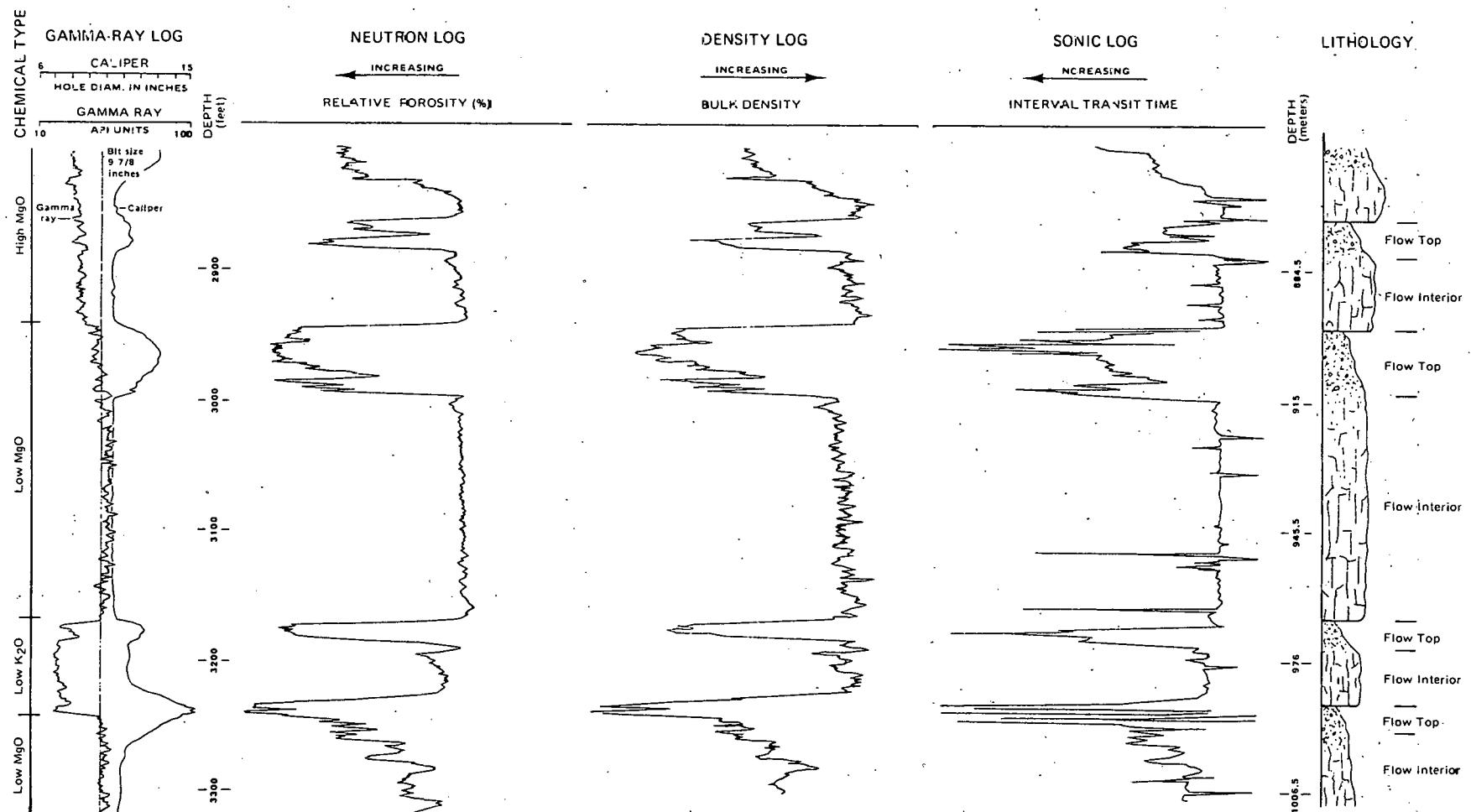
FIGURE 1. Illustrative Wireline Log Response in Columbia River Basalt. Flow tops have higher porosity, lower density, and higher interval transit time than flow interiors. Gamma-ray log is sensitive to chemical types with different potassium percentages.
