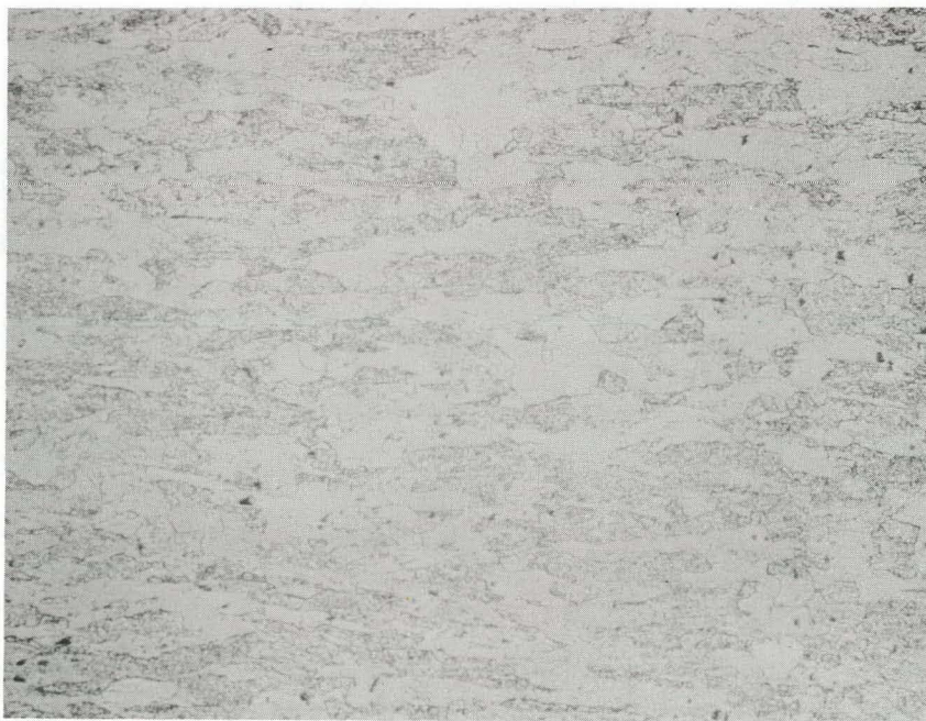
Fig. 36. Recrystallization Data for Drawn Cup. 30-min stress relief at 1350°C. Magn, 100X. Etch: 10% \text{K}_3\text{Fe}(\text{CN})_6
