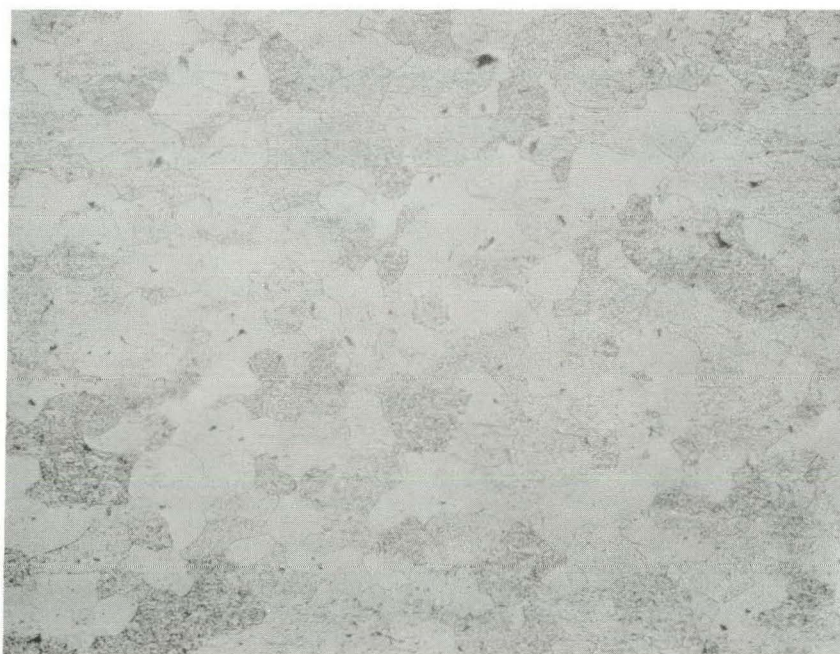
Fig. 38. Recrystallization Data for Drawn Cup. 30-min stress relief at 1450°C. Magn, 100X. Etch: 10% K_3Fe(CN)_6
