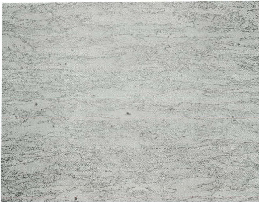
Fig. 35. Recrystallization Data for Drawn Cup. 30-min stress relief at 1300°C. Magn, 100X. Etch: 10% \text{K}_3\text{Fe}(\text{CN})_6
