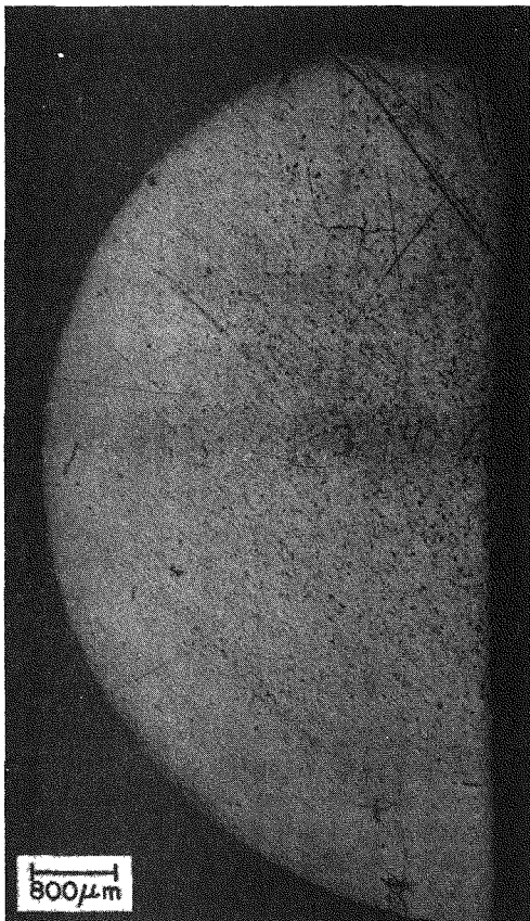
FIGURE 11. Radial Tensile Cracks at the Surface of 91%-TD Pellet MHP 101, As Pressed (Polished Surface)
