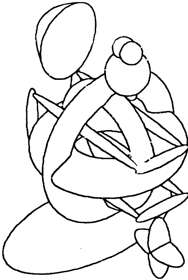
Fig. 5. SABRINA three-dimensional plots of a complicated MCNP geometry. The plot on the right is a cutaway plot of the body on the left. The A and B correspond to the MCNP plots shown in Fig. 4.
