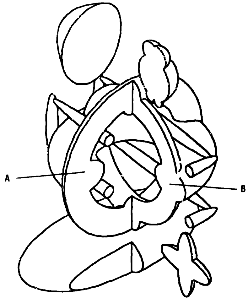
Fig. 5. SABRINA three-dimensional plots of a complicated MCNP geometry. The plot on the right is a cutaway plot of the body on the left. The A and B correspond to the MCNP plots shown in Fig. 4.
