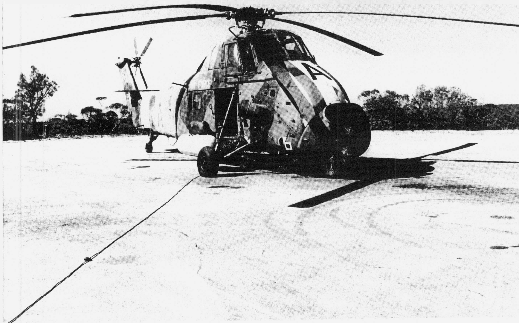
Figure 5. The Royal Air Force Wessex HC.Mk2 Helicopter Shown with the Gamma Ray Detector Pods Installed
