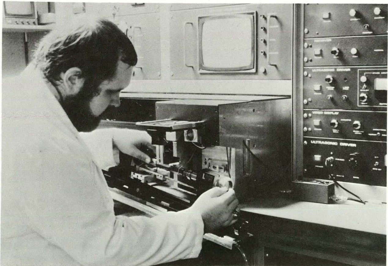
Fig. 14. Photograph of Acoustic Microscope and Stage for Examination of SiC Heat-exchanger Tube Sections.
