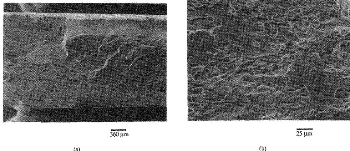
Figure 9: SEM fractographs of GTA weldment in solution heat treated and aged at 160°C for 4 hours: a) overall fracture surface; b) partially melted region.
