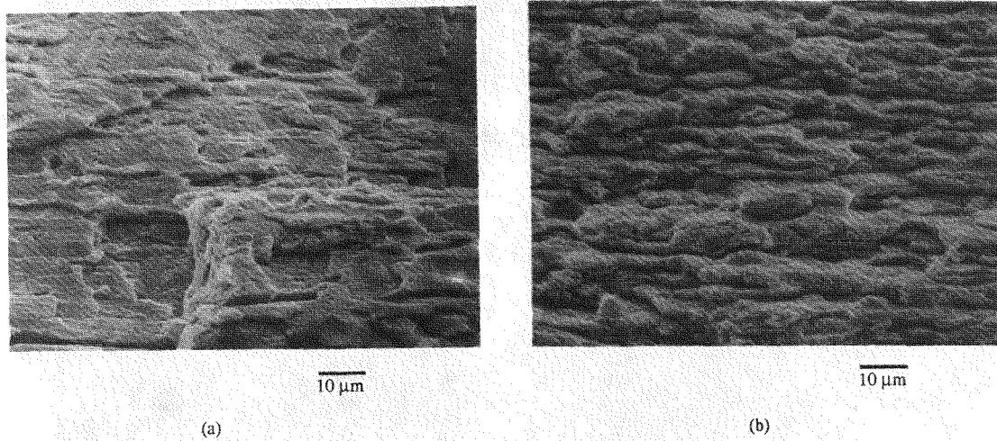
Figure 6: SEM fractographs of base metal: a) aged at 160°C for 16 hours; b) aged at 230°C for 16 hours.
