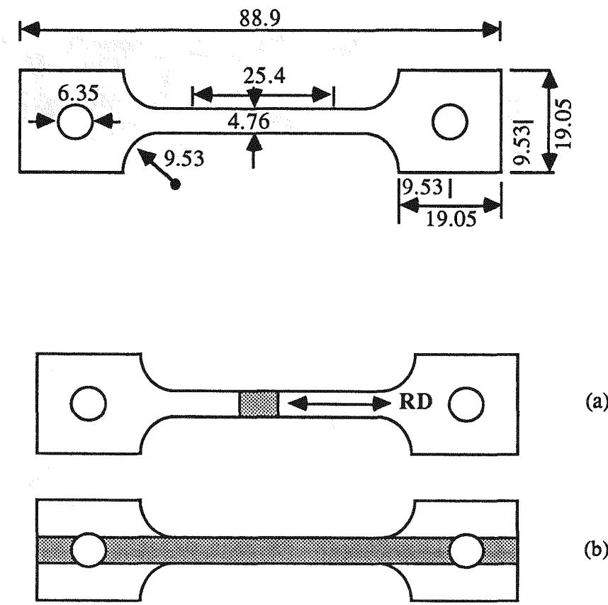
Figure 1: Tensile specimen configuration: a) composite specimen; b) all-weld metal specimen. Dimensions are in mm, and the shaded regions represent the fusion zone.
