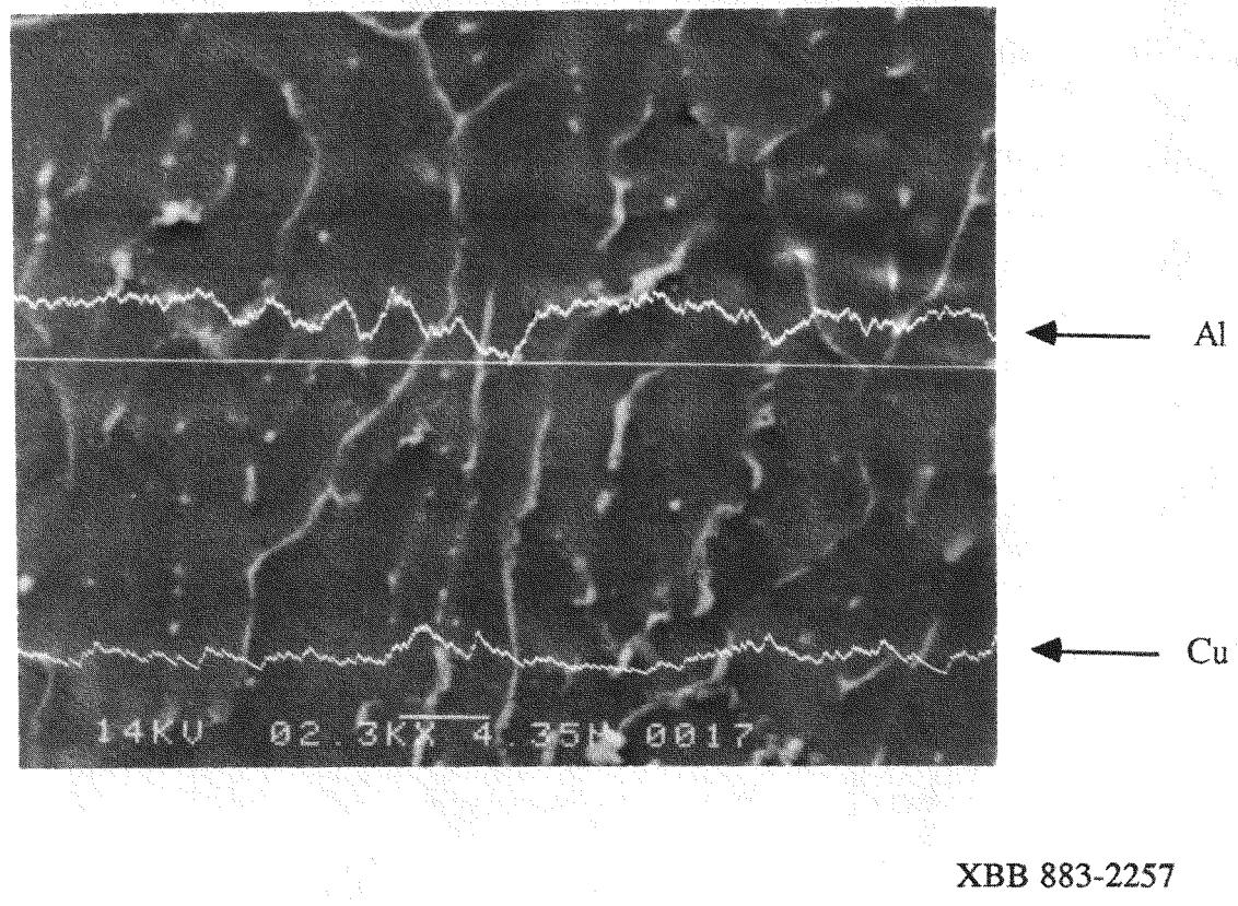
Figure 2: EDX line scan of Al and Cu in the EB fusion zone.
