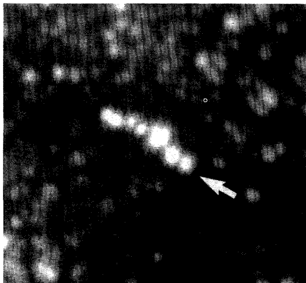
Figure 1. Field ion micrograph of disk-shaped molybdenum carbides in the weld B surveillance material.
