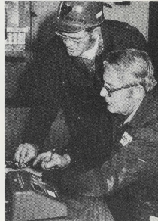
Noise level readings taken with a dosimeter over an eight-hour period at an underground metal mine are averaged on a readout machine by MSHA inspectors.
