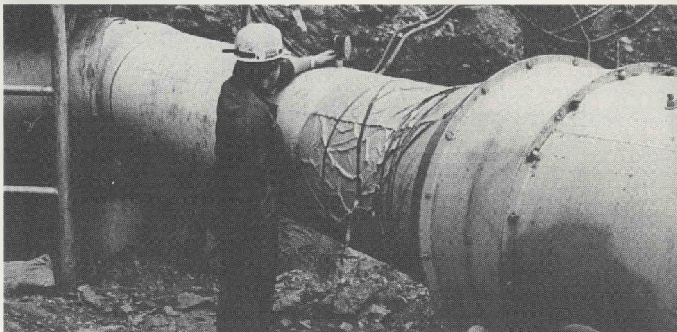
Technical Support provides services to the mining industry in ventilation design, methane and air contaminant control, and in the improvement of mine ventilation systems. In this picture, an air quality test is made in a mine's exhaust ventilation tubing.
