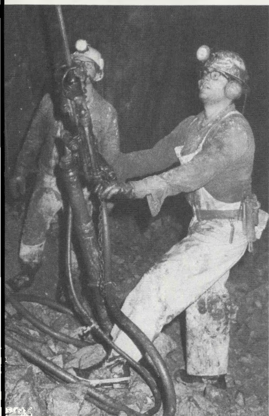
Operation of a jackleg air drill at a molybdenum mine. In recent years, accidents and injuries involving jackleg drills have been significantly reduced through analysis of the hazards in using the equipment, changes in drill designs, and improved operator training.
