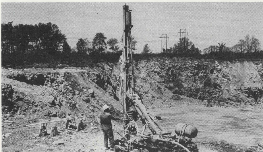
Left, tracked drills such as this one are commonly used at small surface operations to drill holes for explosive shots. The tank on the right of the machine feeds pressurized water to the drill bit to suppress dust which might interfere with the operator's breathing.
