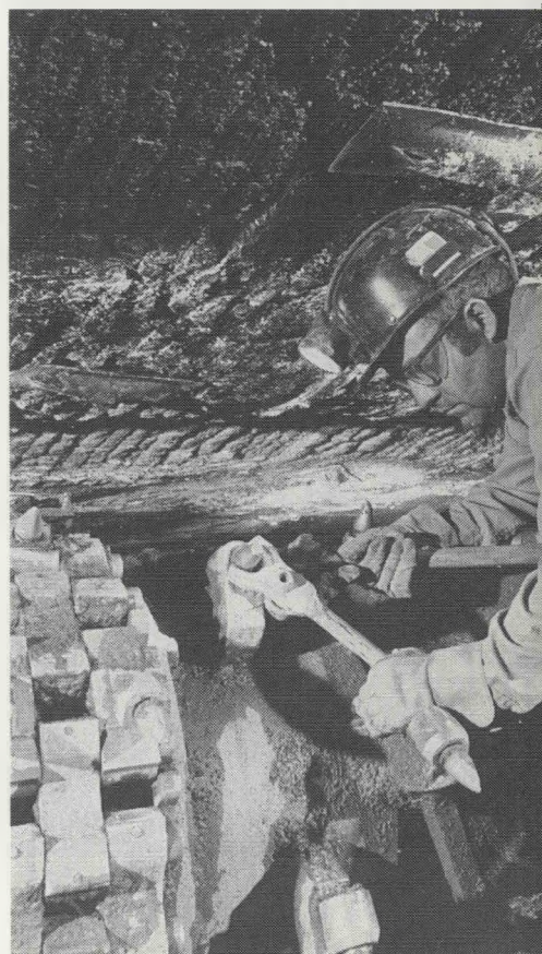
Above, a miner changes a bit on a continuous mining machine in a low coal seam. Roof bolts are visible above the miner's head. Left, an MSHA inspector checks for loose rock as a front-end loader moves through a well-illuminated drift in an underground lead mine.
