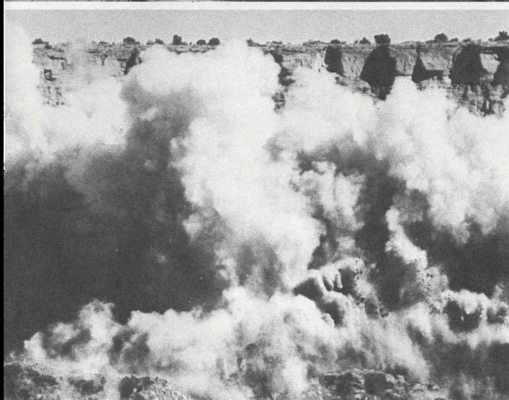
The detonation of explosives at a surface mine sends rock fragments flying. Because "flyrock" has caused deaths and injuries and has destroyed property, careful attention must be paid to clearing people from areas some distance from the blasting site and observing good warning procedures.
