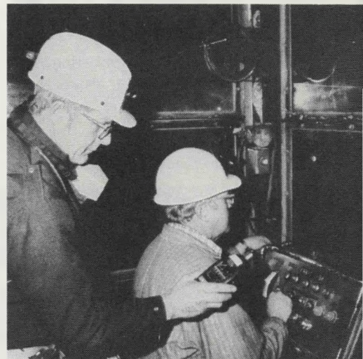
Noise level readings are taken inside a crusher control room at a large metal mill. Built with soundproofing materials, this compartment shields the crusher operator from the deafening process just a few feet away.
