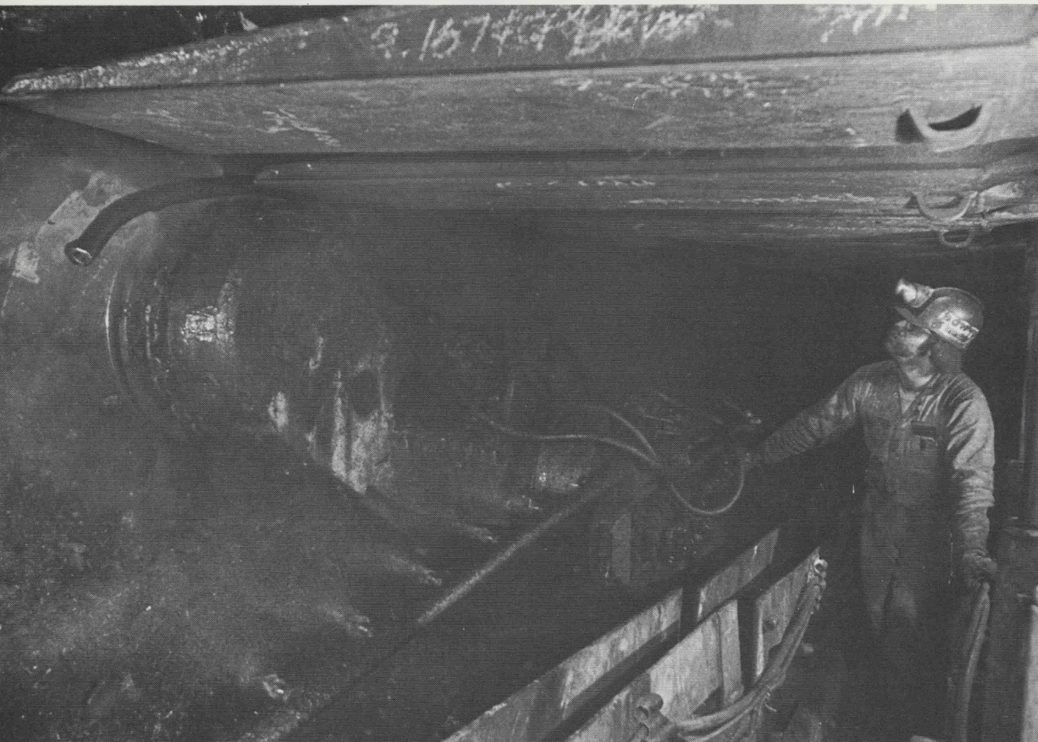
Longwall mining machines, used to mine coal on long, straight faces, are highly productive, but also generate large amounts of coal dust. The water spraying devices attached to this machine reduce airborne dust concentrations.
