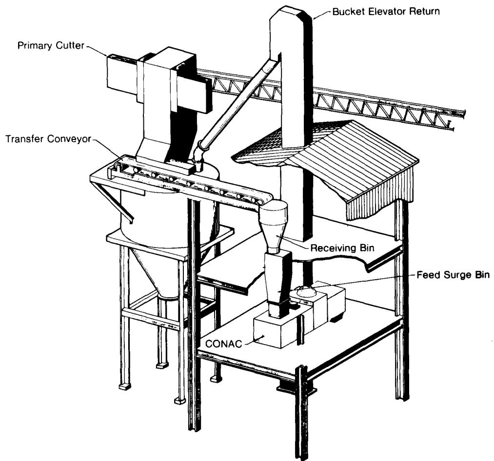
Figure 2-6. CONAC Integrated Into a Typical Power Plant
