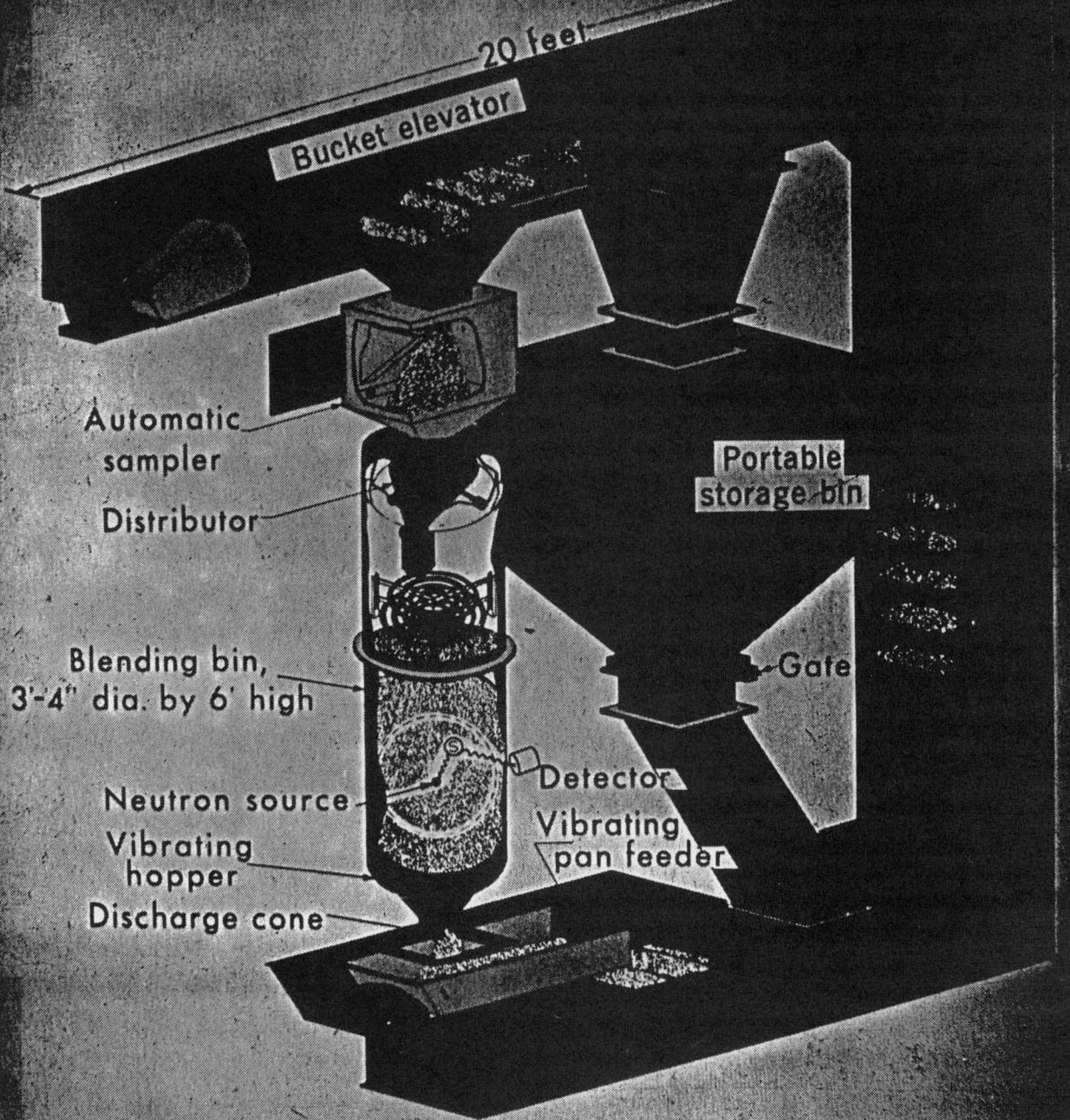
Schematic Diagram of Coal Recycle System.
