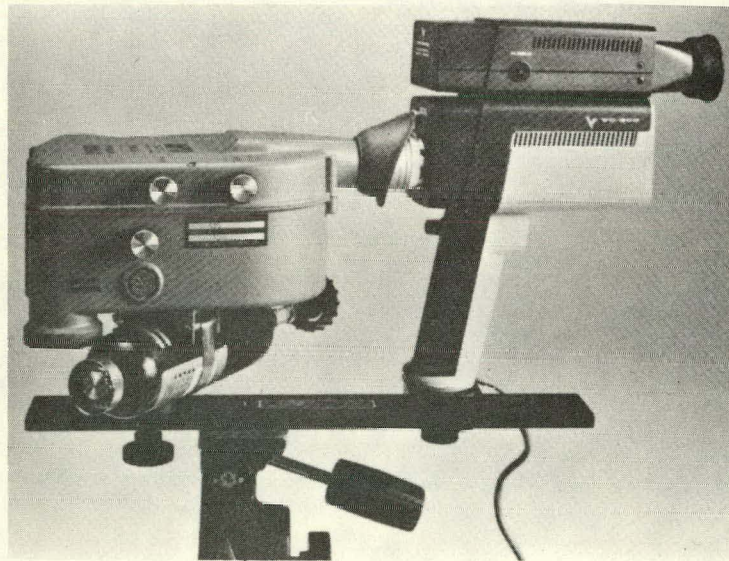
Figure 4. Probeye Infrared Thermal Imager with Video Attachment.
