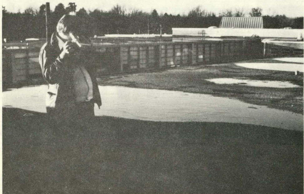
Photograph 8 shows a technologist using an infrared scanner searching for heat loss due to wet or missing insulation.
