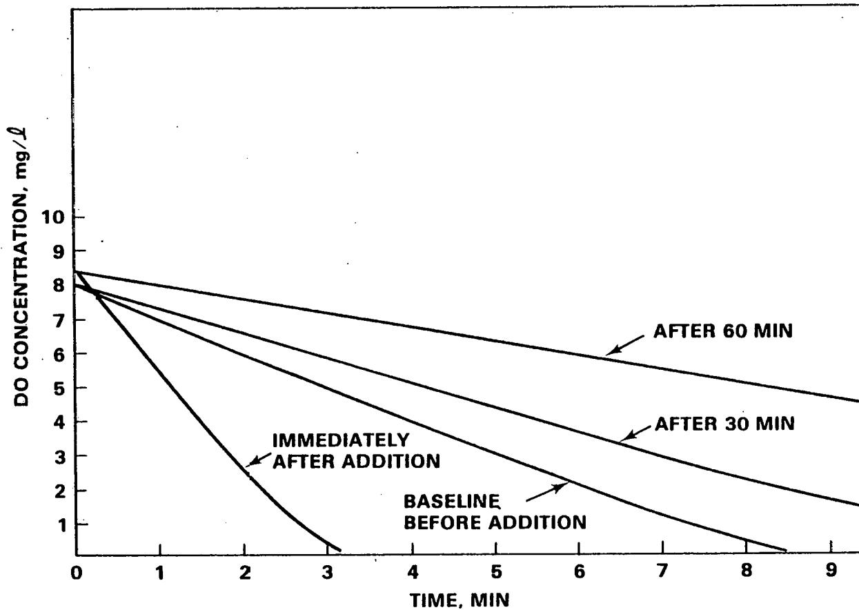
FIGURE 1. Dissolved Oxygen Depletion with Thiosulfate Addition in Activated Sludge
