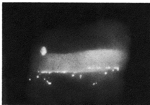
Fig. 4-9. Sudden arc expansion over entire contact, at 4kA, concave bar contact.
