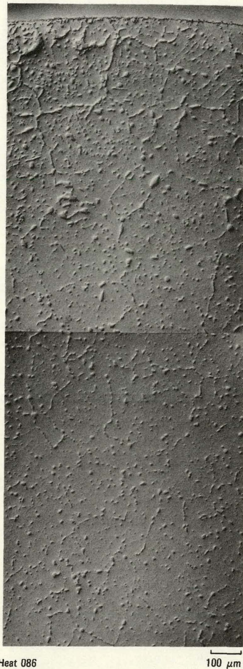
Fig. 16. Optical photomicrograph showing unetched near-surface microstructure of Hastelloy X (heat 086) after 3000-h exposure in controlled-impurity helium at 1000°C. Microstructure shows increased carbide precipitation (carburization) near surface. White layer above surface scale is electrodeposited nickel.
