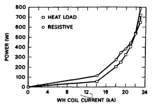
Fig. 6. Resistive power dissipation in WH coil measured resistively and thermodynamically in single-coil extended
