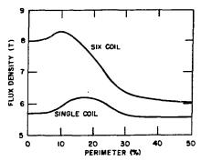
Fig. 3. Field variation from inside turn in middle of straight section of outside perimeter for WH coil.
