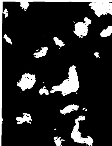
Fig. 1. Dark field TEM (1000 KV) showing cross section of columnar grains in hard, bright electrodeposited chromium.
