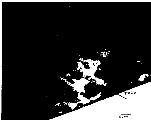
Figure 5. Bright field image of coherent platelets in bulk oxidation specimen.
