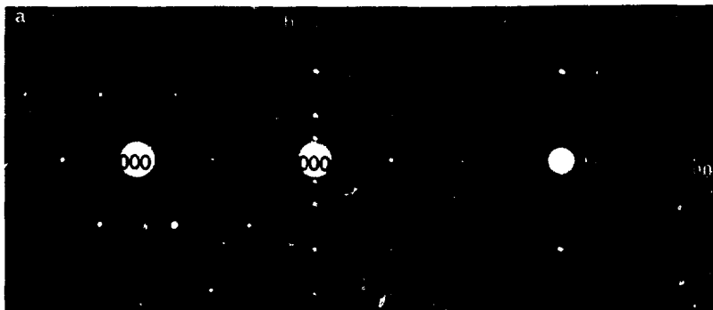
Fig. 2 Electron diffraction patterns for Pd 5 Ce(II) (a) [001] (b) [1-20] (c) [001]
