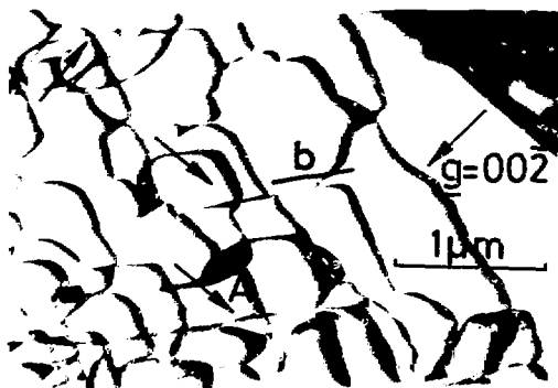
Fig. 4. Dislocation arrangement in glide system (010) [101].
