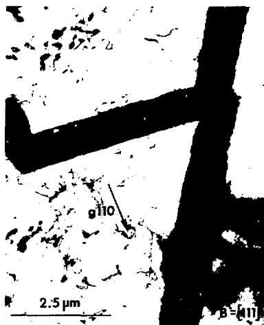
Fig. 5. Fine interfacial line structure observed on \gamma' platelets after in-situ formation at 300°C.
