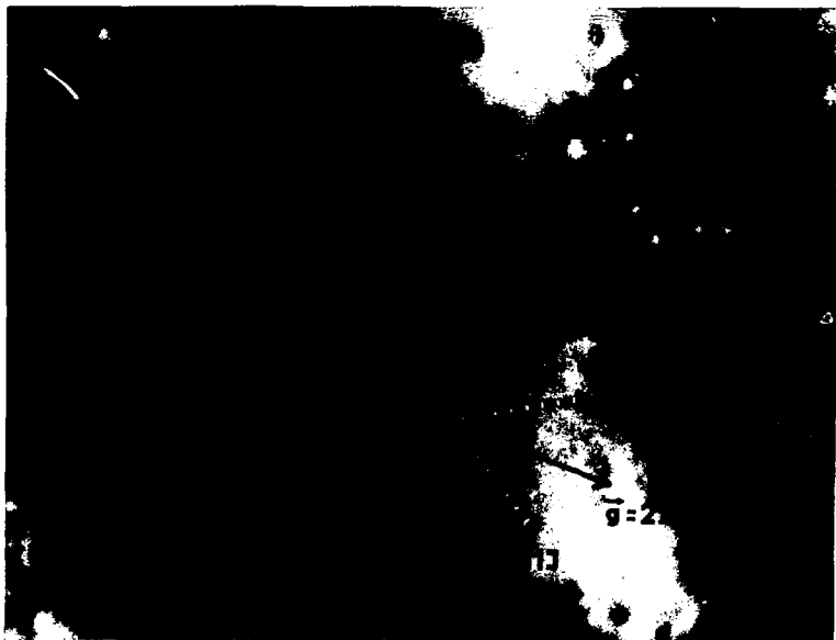
Fig. 1. Black-white contrast of cascade vacancy clusters in Ag irradiated with 20 keV Kr + ions at T < 10 K, dose = 1.2 \times 10^{11} ions/cm 2 , microscopy at T < 10 K with 400 keV electrons, dynamical dark field, g = 220 .
