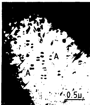
Figures 5(a and b) Ti electron irradiated at \sim 450^\circ\text{C} (723 K) to \sim 0.5 d.p.a. B \sim [0112] , diffracting vectors are indicated. Note the characteristic double arc contrast of the complex loops (marked A) with 2110 .
