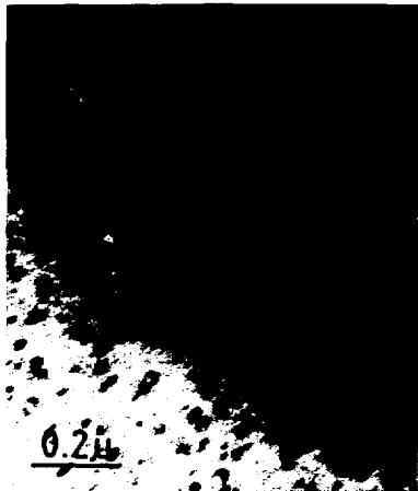
Figure 2 Ti electron irradiated at \sim 400^\circ\text{C} (673 K) to \sim 0.3 d.p.a. \underline{B}\sim \underline{N}\sim[0111] , \underline{g}\sim 10\bar{1}1 .
