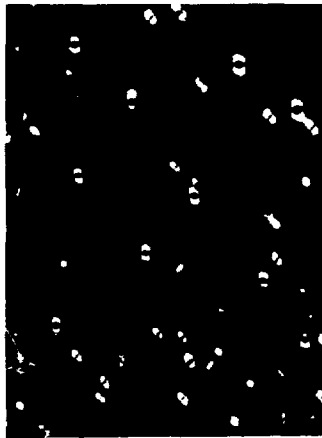
Fig. 2. 1/2 a <110> interstitial dislocation loops in InP irradiated 10 minutes at 350°C with \phi = 3 \times 10^{19} \text{ e.cm}^{-2}.\text{s}^{-1} at 2 MV.
