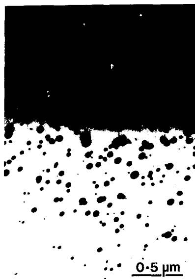
Fig. 3. Micrograph showing unchanged microstructure in thicker regions of foil following in-situ annealing at 725K.
