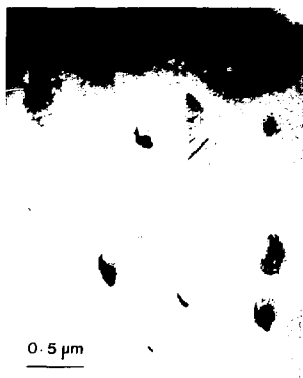
FIGURE 4: B F micrograph showing micro-bend contour in \text{Fe}_{1-x}\text{O} nuclei formed in 1 mPa air at 650^\circ\text{C} for 17 minutes.
