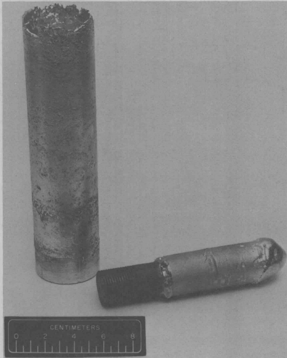
Fig. 5. Consumable arc-melted B-1 ingot on striking pad and electrode stub.
