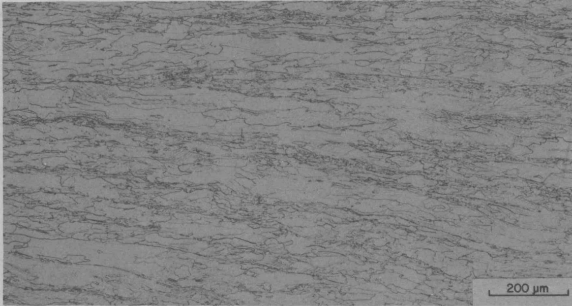
Fig. 15. Longitudinal structure of B-2 rolling billet after being rolled at 1200°C to 74% reduction in thickness.
