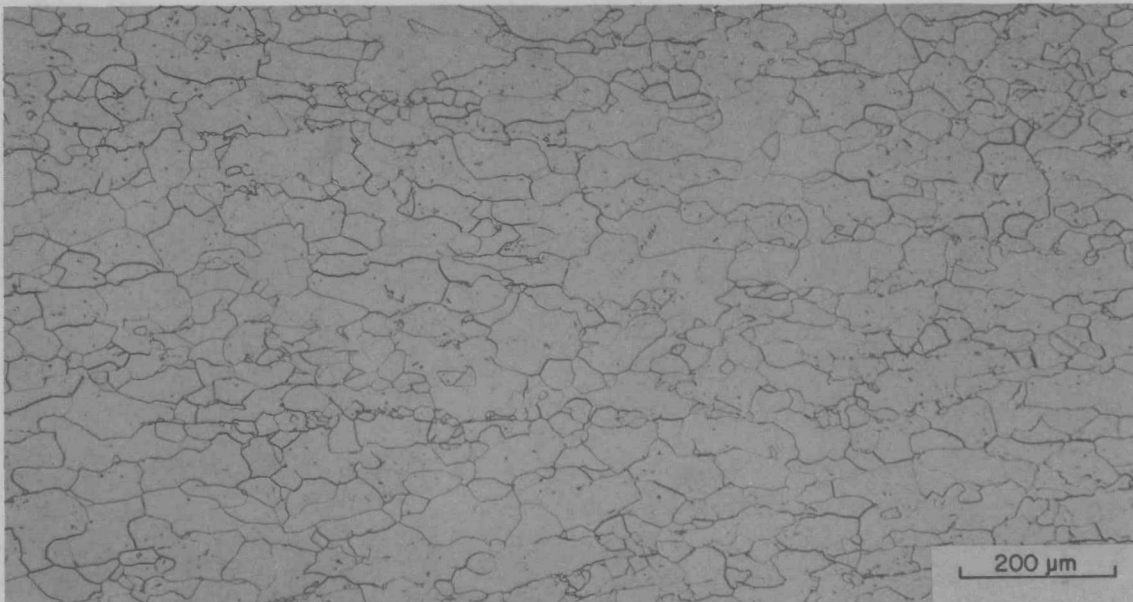
Fig. 16. Longitudinal structure of B-2 rolling billet after being rolled at 1200°C to 74% reduction in thickness and then annealed for 1 h at 1300°C.
