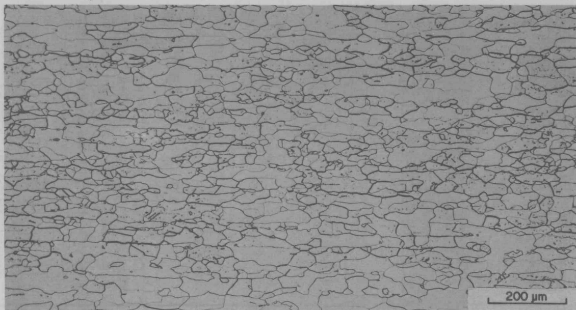
Fig. 22. Longitudinal structure of new-processed sheet recrystallized 1 h at 1300°C.
