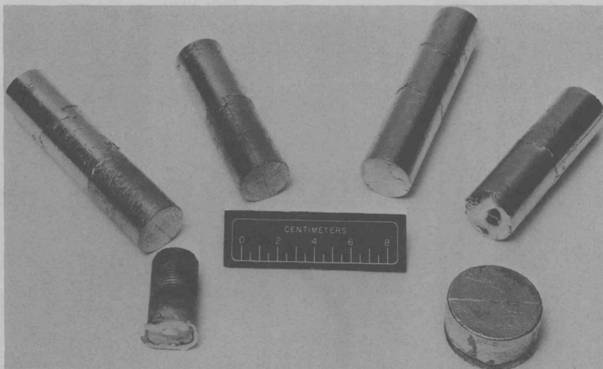
Fig. 3. Arc-melted and drop-cast electrode sections (top four pieces), threaded electrode adaptor (bottom left piece), and striking pad (bottom right piece).
