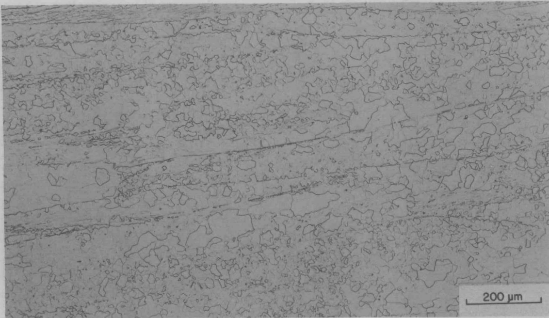
Fig. 9. Longitudinal structure of B-1 bar. The bar was extruded at 1200°C.
