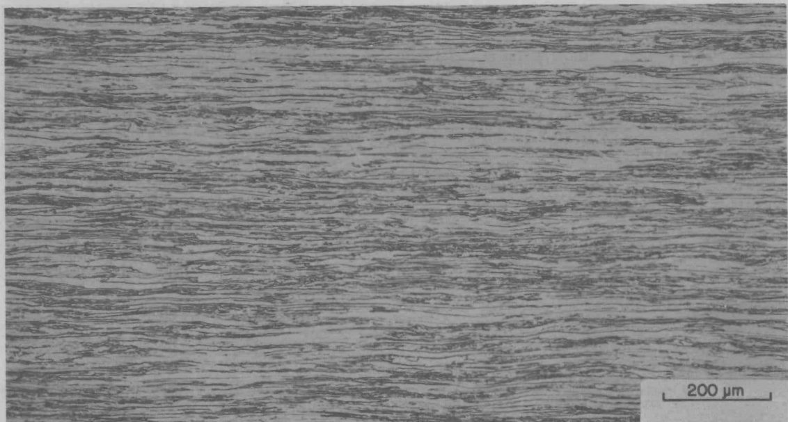
Fig. 19(b). Longitudinal structures of as-rolled B2-5 sheet from central region of the B-2 extrusion.
