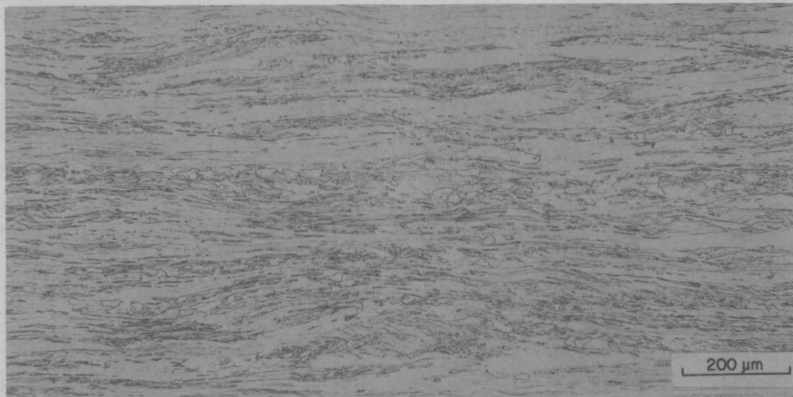
Fig. 21. Longitudinal structure of DOP-26 alloy standard showing maximum permissible recrystallization of 5% of depicted area of sheet.
