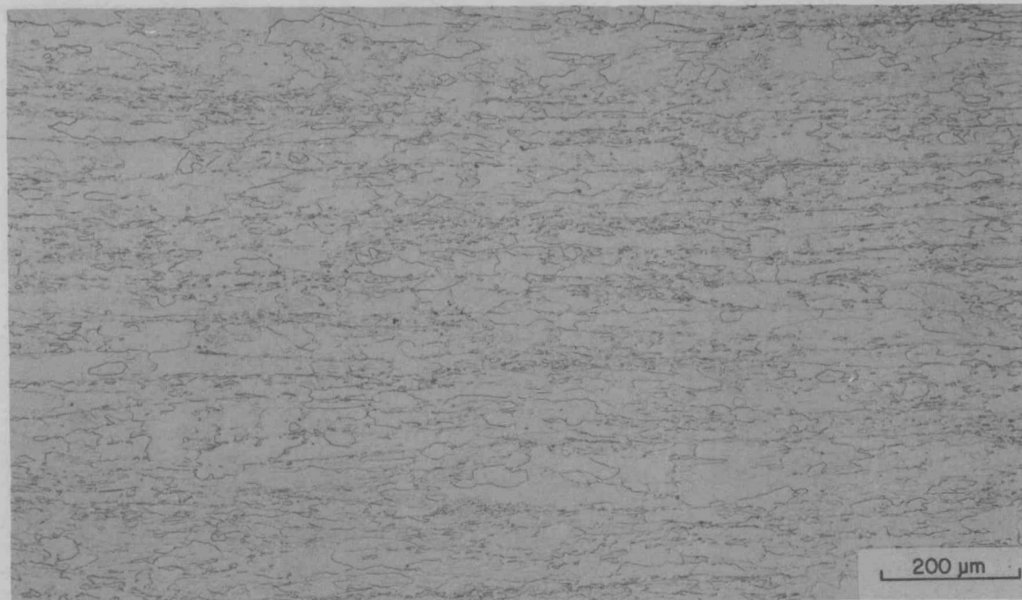
Fig. 11. Longitudinal structure of B-1 rolling billet after being rolled at 1200°C to 74% reduction in thickness.
