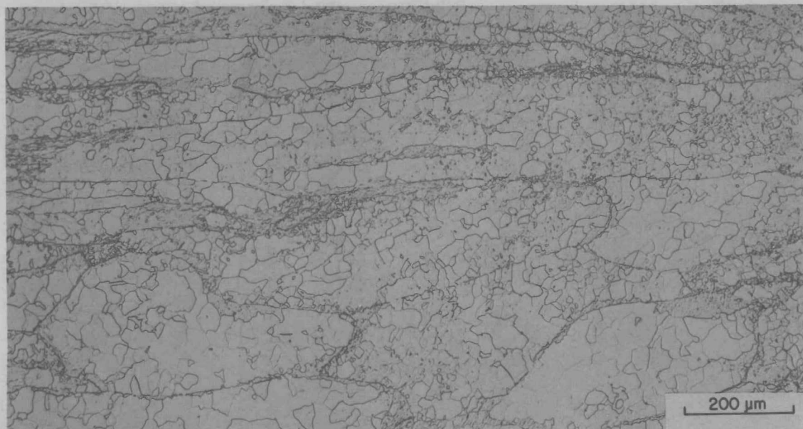
Fig. 14. Transverse structure of B-2 bar that was extruded at 1250°C.
