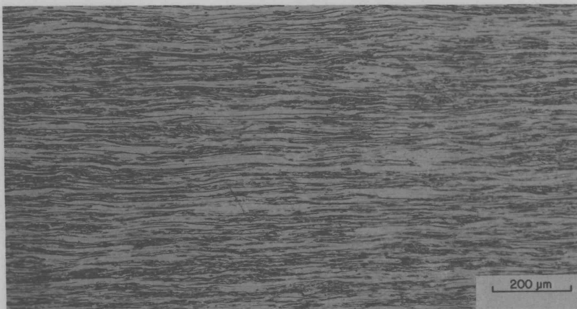
Fig. 18(a). Longitudinal structure of as-rolled B1-1 sheet from nose portion of the B-1 extrusion.
