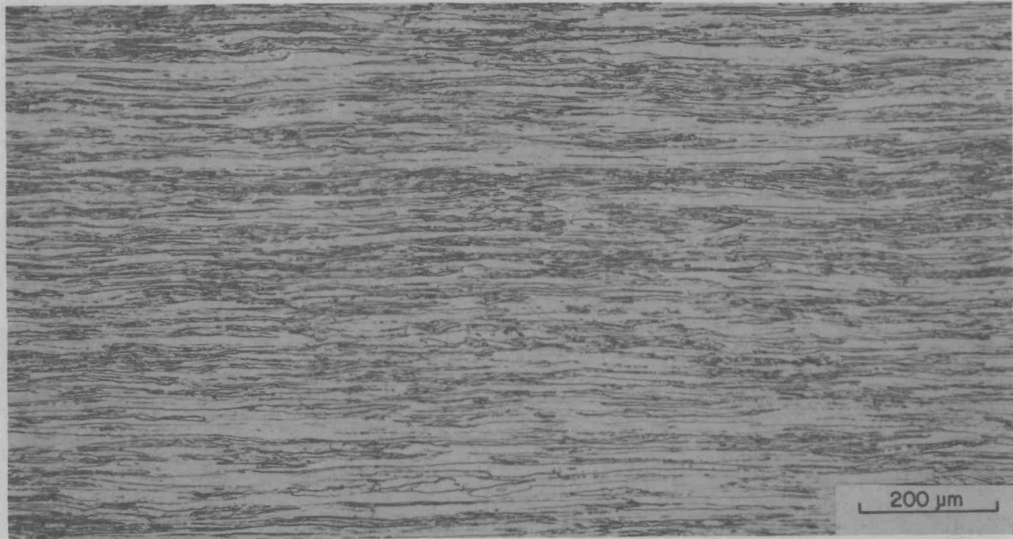
Fig. 19(a). Longitudinal structures of as-rolled B1-4 sheet from central region of the B-1 extrusion.
