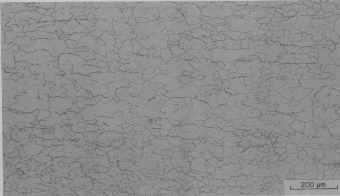
Fig. 12. Longitudinal structure of B-1 rolling billet after being rolled at 1200°C to 74% reduction in thickness and then annealed for 1 h at 1300°C.
