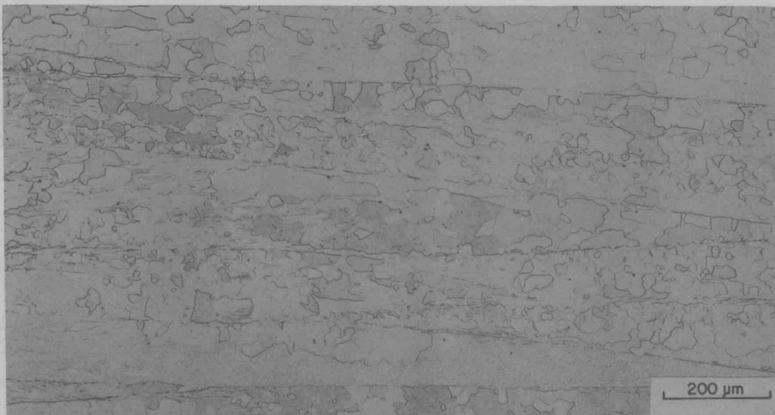
Fig. 13. Longitudinal structure of B-2 bar that was extruded at 1250°C.
