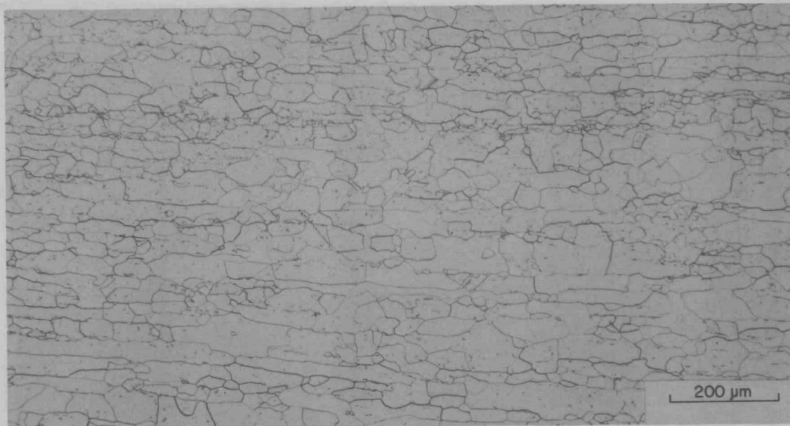
Fig. 17. Longitudinal structure of a B-batch standard-processed DOP-26 alloy ingot after being hot rolled at 1200°C to 74% reduction in thickness and annealed for 1 h at 1300°C.
