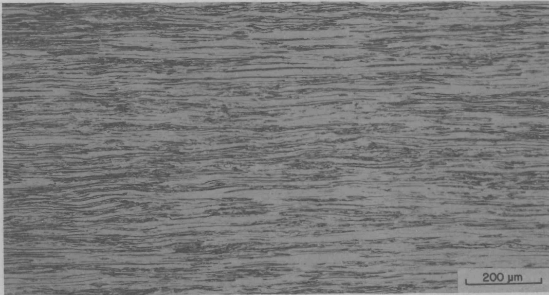
Fig. 20(a). Longitudinal structures of as-rolled B1-7 sheet from tail region of the B-1 extrusion.
