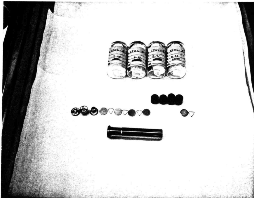
Figure 8-7. Components for emitter fuel loading. The emitter cap is on the far left with fission product trap, fuel holddown spring, heat shields, fuel pellets and fuel support plate arranged to its right.
