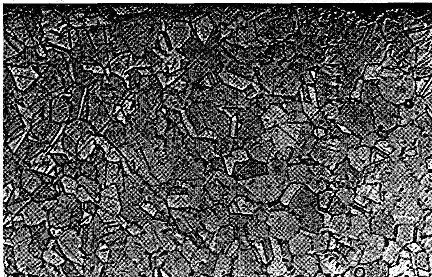
Figure 7. Inconel X-750, SURV-4 ( \text{HNO}_3 - \text{HCl} - \text{H}_2\text{O} etchant)
